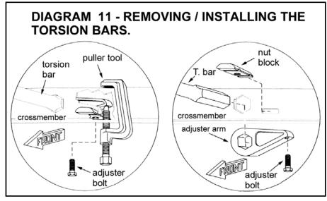
bar, lower control arm, and adjuster arm, then torsion bar rearward into the adjuster arm. Position the special puller tool used during disassembly. Load the puller / bar and install the adjusting bolt and nut block. Use extreme caution while the bar is under load.
