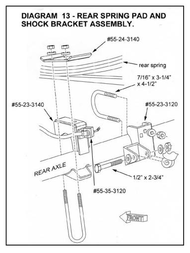
Lower the rear axle to facilitate reinstalling the springs above the axle. Reinstall the springs in the shackles using the factory hardware, but do not fully tighten at this time.
