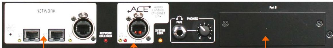
**Control network** 3 port Ethernet switch. Connect laptops, wireless router, link iLive networks, connect external TCP/IP networks, or link to an iLive Surface that does not have an ACE™ port. Control only, no audio.
