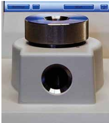
Sample Container with quick release pin
