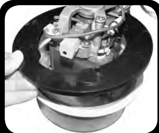
9. Remove ring over top of motor.
