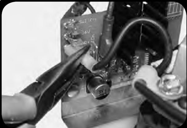
5. Remove horizontal motor connector from BCM.
