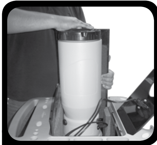
Carefully remove vacuum panel from cart.
