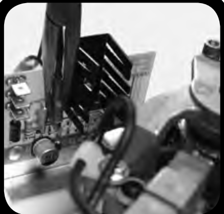
6. Remove thermal switch connector from BCM.
