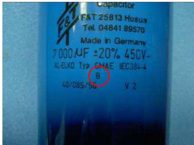
Figure 23: Example of Type B Capacitor
