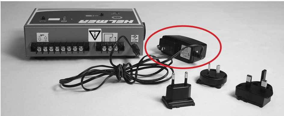
Power supply (circled) with adapters.
