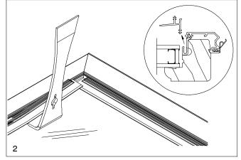
CAUTION: If reglazing sash installed in unit frame, assistance will be necessary while attempting the following procedures. Glass may fall out if not held in place from the exterior while cutting the interior glazing seal.
