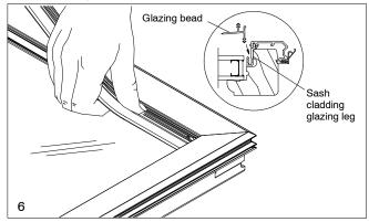
10. If applicable, install aluminum glazing cap, starting with the rails first. Slide cap flush with sash cladding and tap onto vinyl glazing bead connecting barb with a rubber mallet as shown in illustration 7. Install stile glazing cap in the same manner flush against rail cap.
