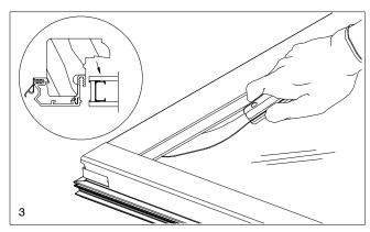
5. Clean all remaining glazing sealant or adhesive tape residue from glass rabbet. It is very important that glazing surfaces are free from debris to ensure a proper seal on new glass.
