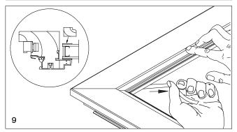
14. When all bead is in place press down firmly and nail to sash 1" from each corner and every 4"-6" (102-152) with 1 1/4" 16 gauge brad nails. Be careful not to angle nail toward glass. See illustration 10.
