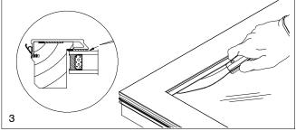
6. Clean all remaining glazing sealant from cladding and wood bead (if it is to be reused). It is very important that glazing surfaces are free from debris to ensure a proper seal on new glass.
