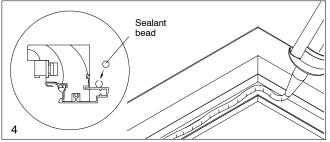
For clad Casemaster Round Top units, position sash frame with interior side up. Apply 1/2" glazing tape flush with cladding on glazing rabbet. Remove paper backing from tape. Apply a 1/8" (3) bead of sealant behind tape. See illustration 5.
