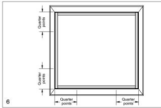
11. Dry fit replacement wood bead to ensure a proper fit. Some trimming may be necessary. On units that use glazing tape DO NOT remove paper backing. Begin with the shortest pieces first then install the longer pieces. On Round Top units install radius wood bead first then the bottom rail bead. When all wood bead components fit correctly remove and proceed to next step.
