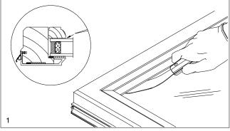
3. Starting at the center of each piece, remove the wood bead by cutting between the bead and sash with a stiff bladed putty knife, prying the bead away from the sash. See illustration 2.
