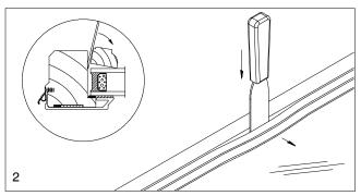
CAUTION: Be careful not to mar the sash while removing the wood bead. If reusing take care not to damage or split wood bead during removal.
