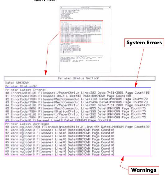
You can also obtain report of the System Error and Warnings through the DesignJet System Maintenance Tool.
