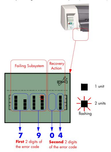
Refer to Page 2-14 for an explanation on the construction of the Error Codes and Warnings.
