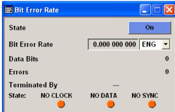
The top section indicates if the bit error rate measurement is active and displays the results and current status of the measurement.
