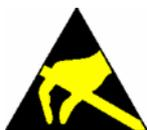
To avoid damaging the electronic components of the EUT (Equipment Under Test) due to electrostatic discharge produced by contact, the use of appropriate protective measures is recommended.
