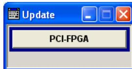
After a firmware update it is occasionally required to update the PCI-FPGA also. This is enabled in the **Update** dialog.
