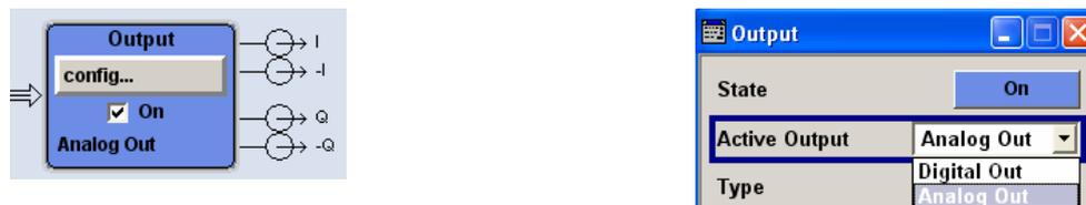
In the upper part of the dialog, the output (analog or digital) is selected and activated. The dialog differs depending on the selected output.
