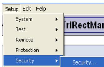
The menu is divided into the Change Security Password section and the Security Settings section. In the password section the passwords for securing a controlled access to the instrument are defined and changed. In the security section the remote interfaces are enabled and disabled.
