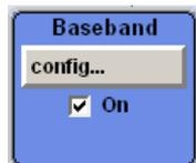
In the check box  **On**, the respective function can be quickly activated/deactivated with the **[Ctrl] + [T]** key combination. After activation, the block is displayed in blue.
