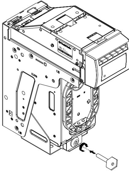
Pressing the lever (located to the right) releases the Cassette for easy removal.
