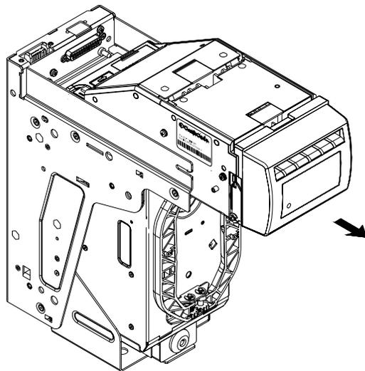
**Step 3.** Remove the Dummy Card (or Memory Card) from the Memory Card slot of the Validating Head (please see diagram below).
