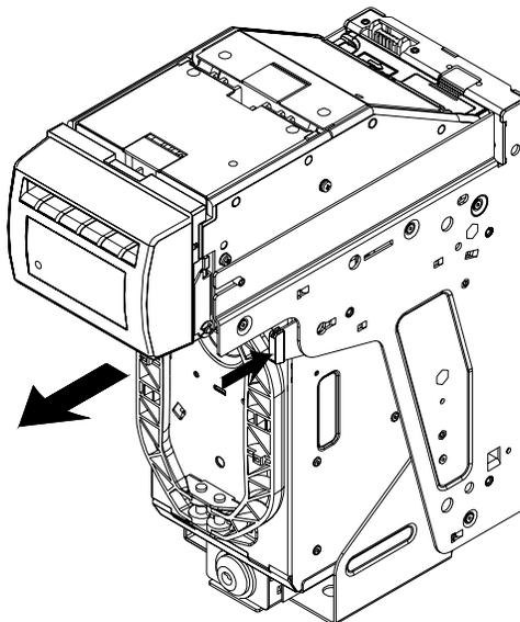
To replace the Cassette, close the Cassette cover, insert the Cassette into the FrontLoad frame, and turn the key to lock the Cassette back in place.
