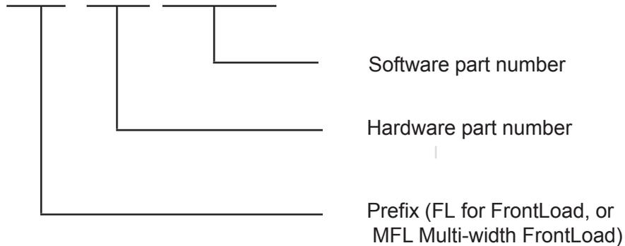
The Prefix defines the device class. Here FL means “FrontLoad Bill Validator” and MFL means “Multi-width Front Load Bill Validator” (i.e. with a centering mechanism in the Validating Head).
