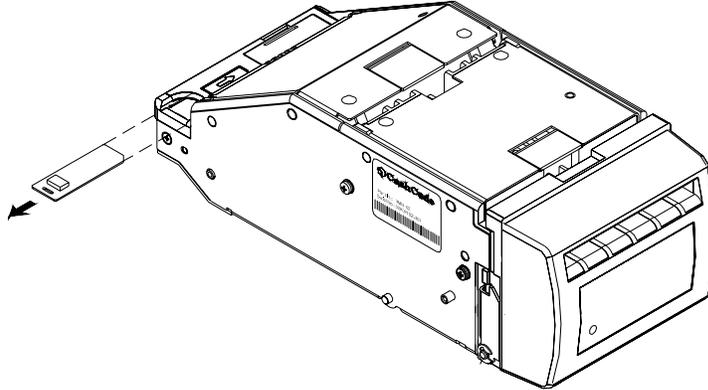
**Step 4.** Insert the new CashCode Memory Card into the Memory Card slot of the Validating Head (please see diagram below).
