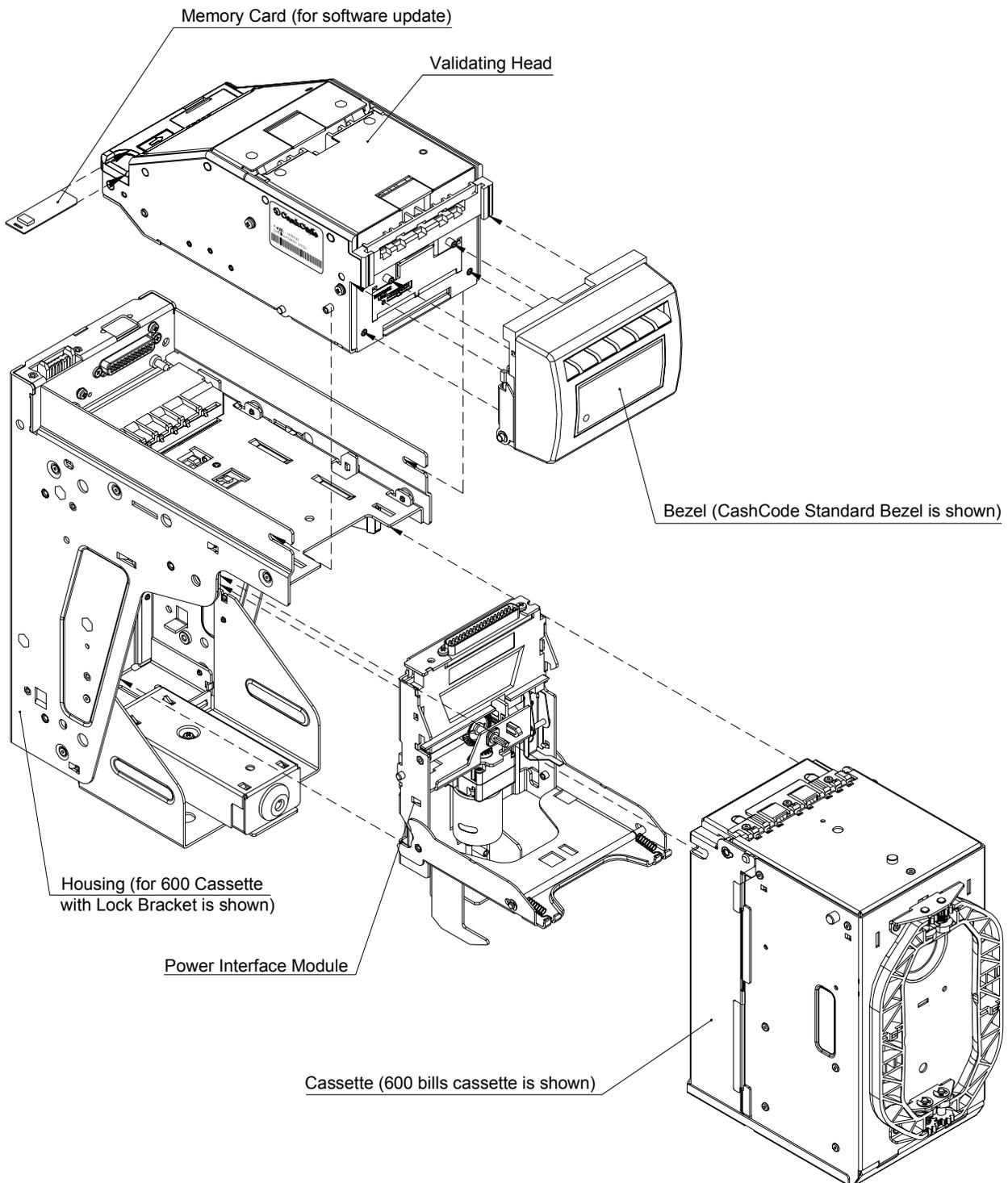
The FrontLoad bill validator is designed accommodate bills 62 to 82 mm wide and 125 to 172 mm long – which encompasses most currencies.
