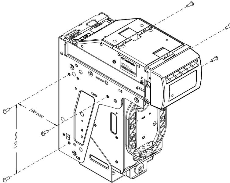
If the position of the mounting screws is different than the position of the mounting holes provided in the target equipment, then additional frame mounting components may be required.
