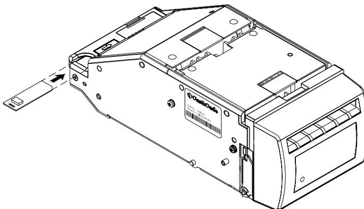
**Step 5.** Insert the Validating Head into the Housing.
