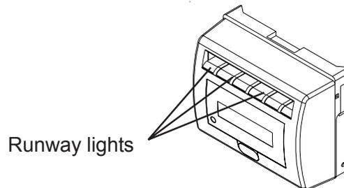
**CashCode Bezel with runway lights and digital display.** In addition to runway lights, a digital display of 2 lines (16 characters each) is available.
