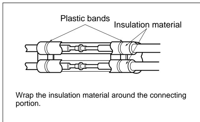
**9. Set the pipings and the connecting cable to the back of the chassis with the tubing holder.**
