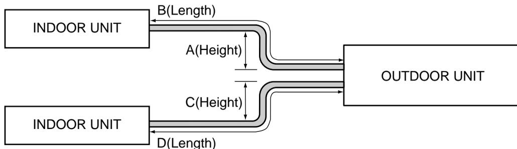
\*\* A, B mean indoor unit higher located than outdoor unit.
