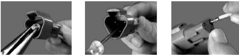
Figure 3-13. DT/DTP Contact Removal
