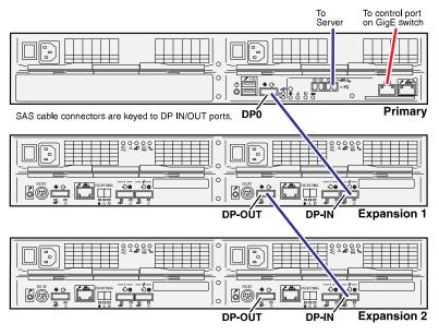
NOTE: Do not connect the controller MNT port. It should only be used with a PC in a peer-to-peer connection for diagnostics purposes.
