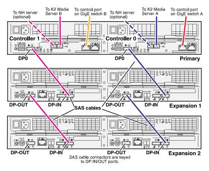
NOTE: Do not connect the controller MNT port. It should only be used with a PC in a peer-to-peer connection for diagnostics purposes.
