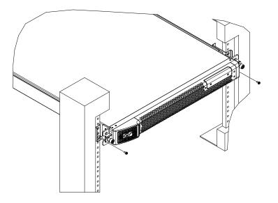
Install a screw in the bottom hole of the bracket on each side. Do not attempt to install a screw in the top hole of the bracket.
