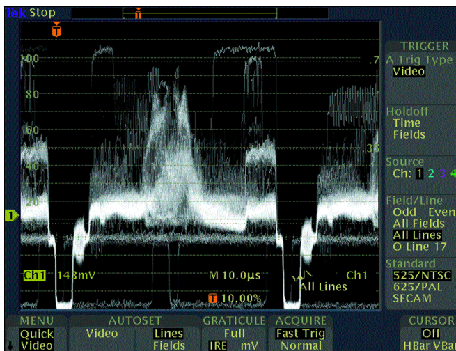
Figure 1. DPO technology brings out vivid waveform detail on the IRE graticule (available with video module).
