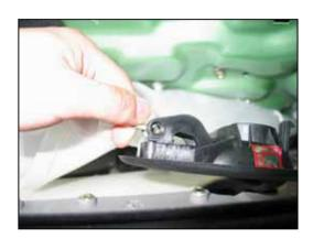
(6) Disconnect the wire harness plug of central lock main switch from the rear of door inner door panel, and then take out the base plate of door handle.
