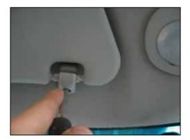
(3) Loosen 3 handles on the roof panel.
