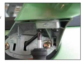
(4) Loosen the harness connector of the mirror from the door inner panel; take out the rearview mirror assembly.
