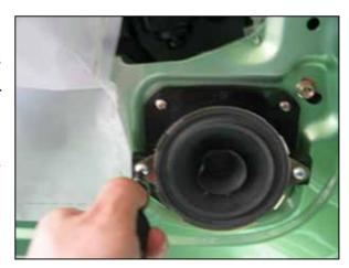
(3) Remove the horn plug, take the horn out.
