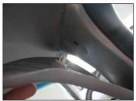
(2) Loosen bolts on the sun shading panel with screwdriver.
