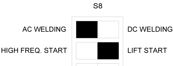
FIGURE 15 - LIFT-START START MODE AND AC WELDING
