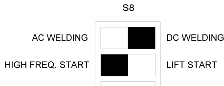
FIGURE 14 - HF START MODE AND DC WELDING
