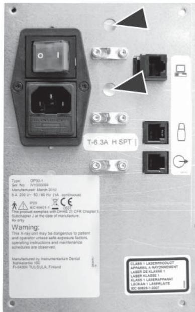
2. Route the cable that comes from the external exposure switch through one of the holes in the board mounting plate assembly to the rear of the assembly.
