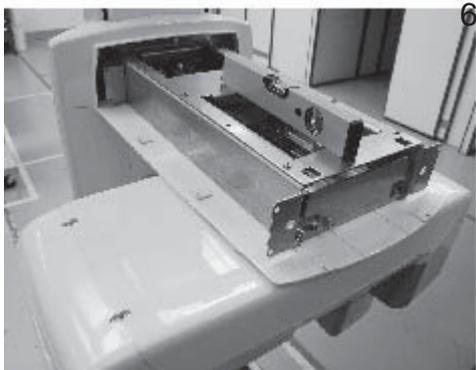
Make large adjustments by moving the the base of the column backwards or forwards.
