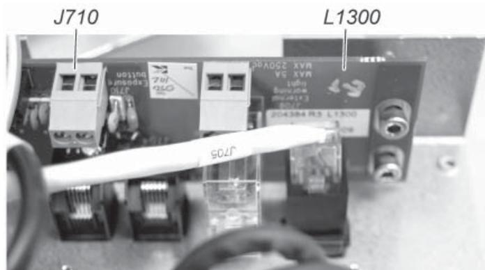
4. Replace the board mounting plate assembly and secure the cable that goes to the remote exposure warning light in position under one of the cable clamps.
