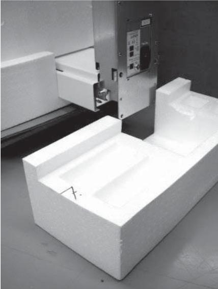
5. Fold down the end of the box that is nearest the hinged section part of the column and then slide the unit over the edge of the pallet so that you can access the underside of the hinged section of the column.
