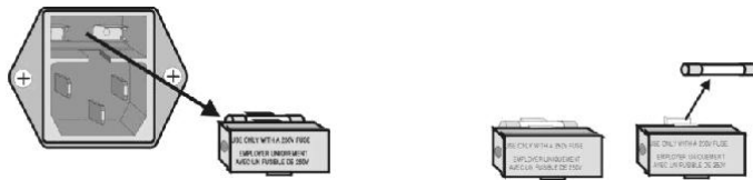
[ Replacing the Fuse ]
