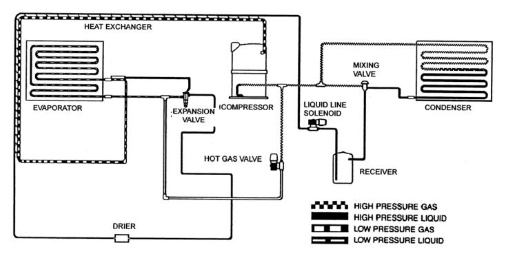
The Remote Refrigeration System is shown in the above diagram. During the freezing cycle, high temperature and high pressure liquid refrigerant is directed from the condenser through a mixing valve, receiver, liquid line solenoid heat exchanger and a filter drier. The expansion valve meters refrigerant to the coils on the back of the evaporator.
