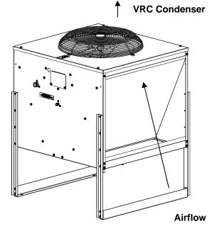
The remote condensers incorporate the mixing valve in the condenser. This configuration allows up to a 100 foot calculated remote line set run. Reference the diagram below to calculate the maximum 100 foot line set run.
