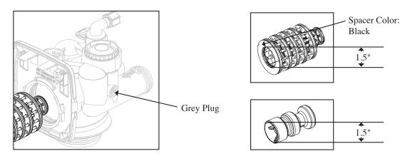
WS1.25 with 32mm Distributor Tube Opening Identification
