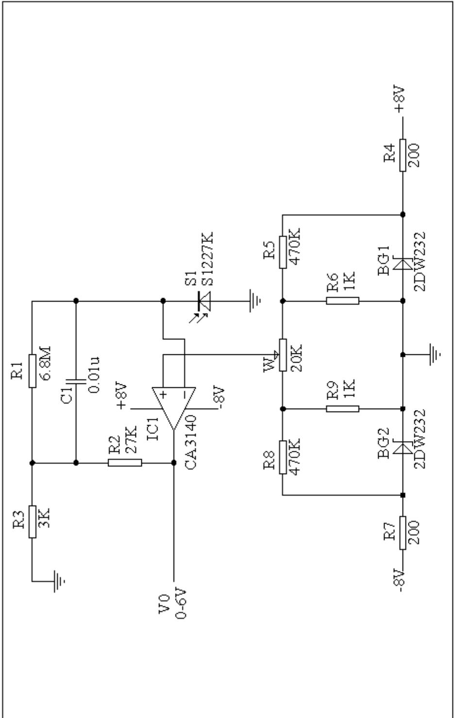
Fig5.3.1 Circuit Diagram of Amplifier
