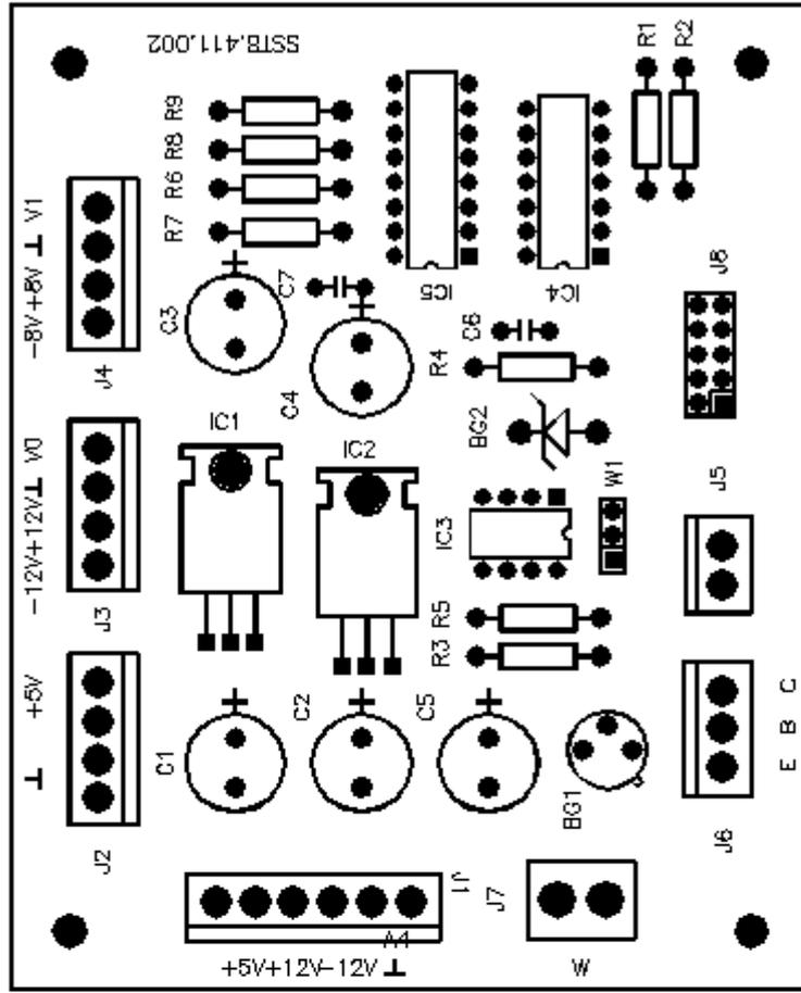
Fig5.1 PCB Arrangement of Power Supply
