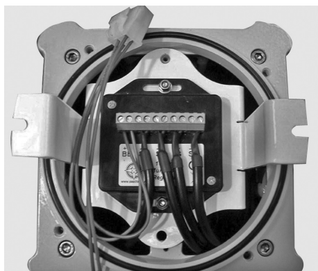
SL10 AMP Regulator shown when correctly fitted
