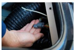
2. Disconnect this connector, and plug the SBT Yamaha adapter cable light gray connector into the mating connector on the Waverunner harness:
