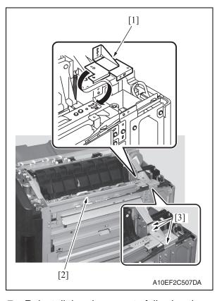
6. Remove the plate [1], and remove the punch kit [2].
