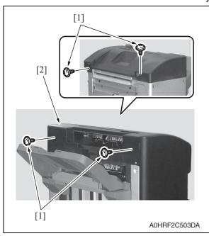
2. Remove four screws [1], and remove the finisher upper cover [2].
