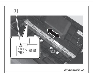
Move the punch unit forward or backward for adjustment referring the mark-off line [1]. Blank Page
