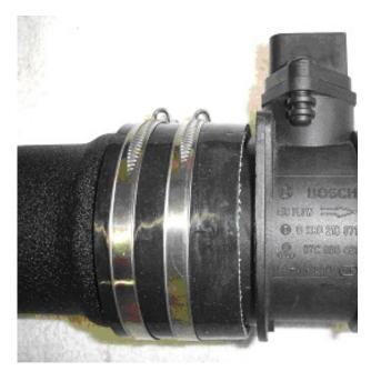
Clamp the provided K&N filter to the end of the bracketed pipe. Making sure the coupler is completely covered.
