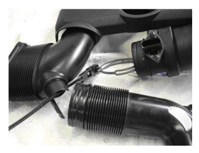
Unscrew and CAREFULLY REMOVE MAF HOUSING. (\*\*\*If the MAF is dropped or damaged, your car may not start.) The MAF housing will be used later on in these instructions
