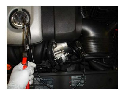
Disconnect the second spring clamp and remove plastic flexi duct from MAF housing.
