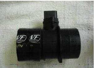
Slide the other side of the MAF into the swedged end of the bracketed pipe. The arrow on the MAF must be pointing towards intake manifold (direction of air flow).
