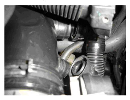
Unclip ambient temperature sensor and remove the spring clamp then pull off engine cover.
