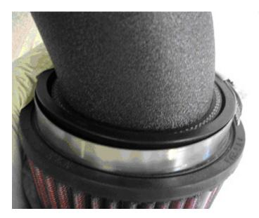
Without fully tightening any hose clamps (apart from K&N filter), wiggle the filter end of the bracketed pipe through the gap between the right headlight and the chassis. Do not bolt the bracket down until the intake pipe is fully connected.
