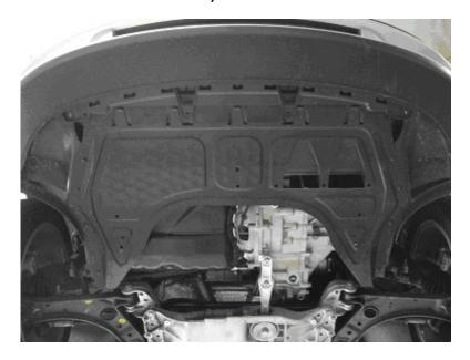
Remove the under tray using a T20 torque driver. There are eight screws. There are two bolts that emerge from the chassis on the driver's side. Push the heat shield into position shown. The plastic trims and shield may need to be twisted slightly to allow the VF shield to get into postion.
