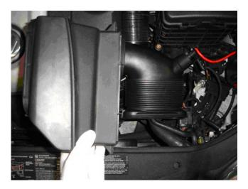
3. Carefully remove the secondary air injection and crank case vent "quick connectors" from the MAF flex duct by squeezing the outer ring between your index finger and thumb. Unclip the large spring clamps around the flexi duct that secure it to the throttle body and the MAF. (\*\*\*Note: Take caution as this hose is very brittle and can crack easily if it is flexed excessively!) (WEAR EYE PROTECTION WHEN REMOVING SPRING CLIP)
