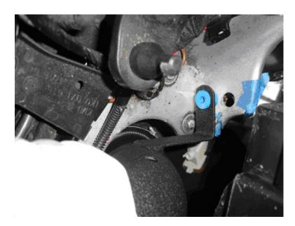
Now slide the pipe that attaches onto the intake manifold as shown. Do not connect the crank case vent or the secondary air injection until the intake is in the desired position.
