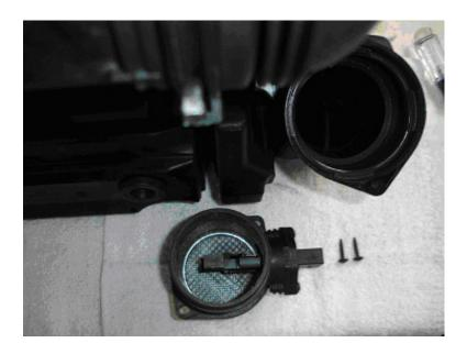
Apply silicone lubricant to coupler at the end of shorter pipe and place over MAF housing (the side without a protective mesh).
