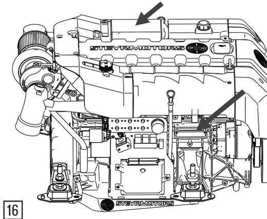
**17** The model and serial number of the marine gearbox is located on the marine gearbox housing as illustrated.
