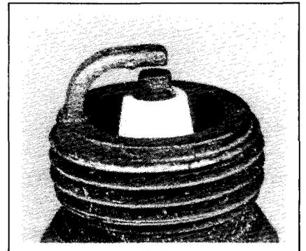
**Chalky White Deposits:** Chalky white colored deposits indicate overheating. This condition is usually accompanied by excessive gap erosion. A clogged grass screen, clogged cooling fins, and lean carburetion are some causes of over-heating.
