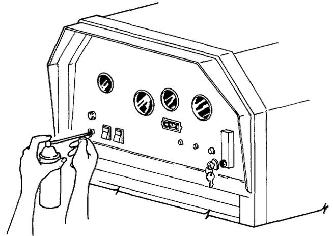
Spray lubricant into blower lube port for 3 to 5 seconds, then immediately shut off machine. Use only LPS 1 or Pennzguard moisture displacing lubricants.
