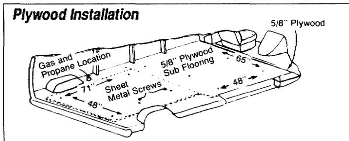
SECOND, select the appropriate color astroturf to match your van and cover the plywood and staple in place. A standard van requires a piece 6 feet by 12 feet.
