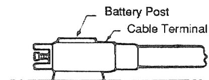
Poor contact at the battery cable connections is often a source of trouble. Make sure battery cables are in good condition and that contacting surfaces are clean and tightly connected. Do not reverse battery leads. Use recommended battery tools when disconnecting leads to avoid mechanical battery damage.
