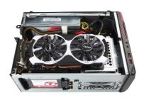
Step 4. Press the catch at the end of the PCIE slot downward to unlock the graphics card. Uninstall the graphics card and watch out to the power cable attached to the graphics card.
