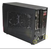
Step 2. Remove the cover carefully. Keep the screws and the cover for later use.
