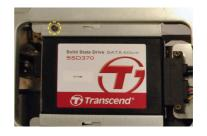
**Step 2.** Press and slide the SSD module by the direction as the figure shows.
