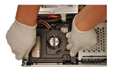
Step 4. Remove the fan power cable and put the fan & adapter module at a save place.
