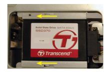
Step 3. Unscrew the 4 screws fixing the SSD. Remove the SSD carefully from the tray and set it aside for later use.
