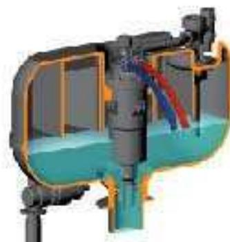
C. Air pressure acts as a powerful piston to drive the water from the vessel into the bowl
