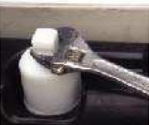
Step 6. Using the tool provided engage the interlocking teeth and rotate the FVC counter clockwise  $\frac{1}{4}$  turn. Then lift the FVC up removing it from the vessel.
