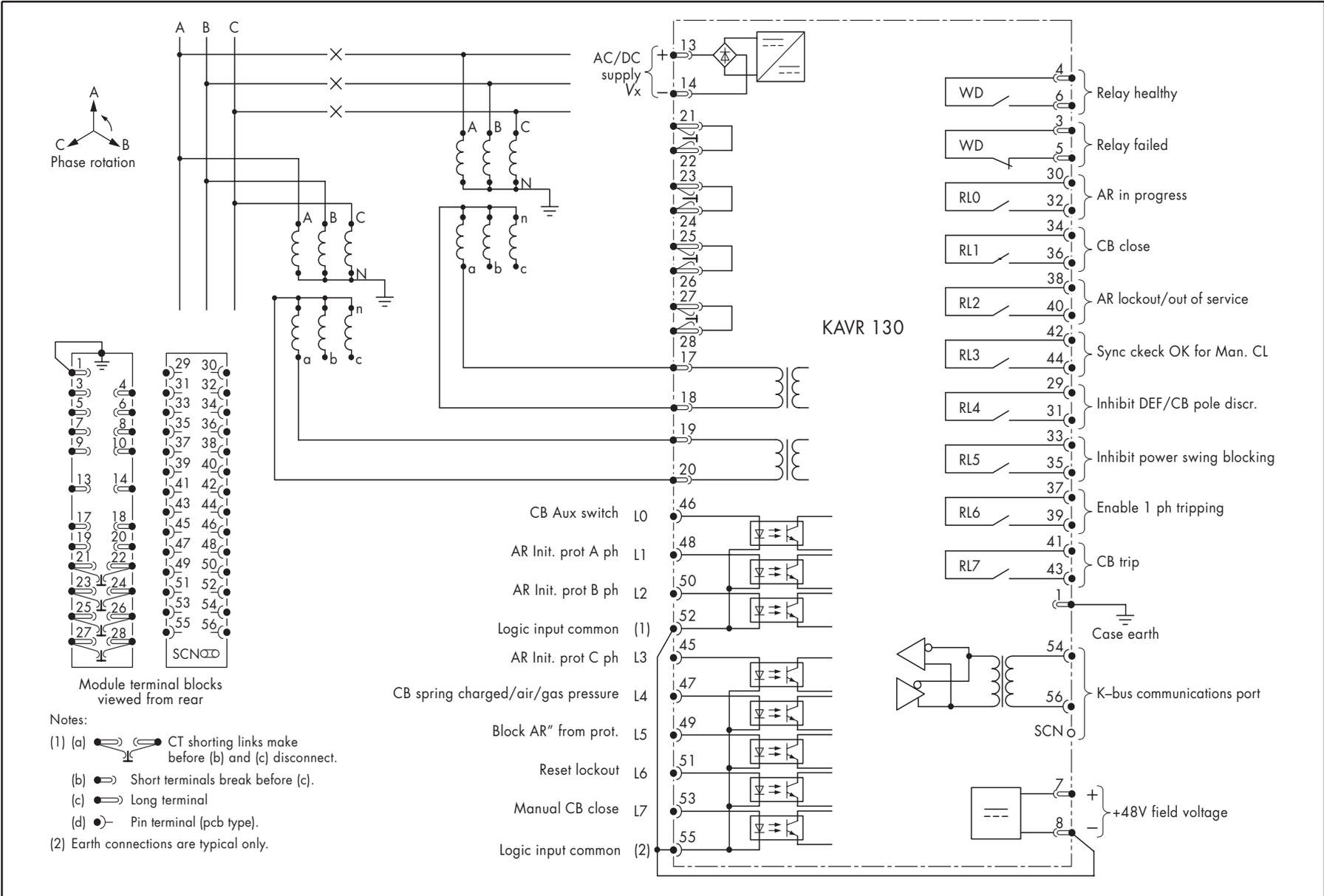
**Figure 31. Typical application diagram: Midos auto-reclose and check synchronising relay type KAVR 100**
