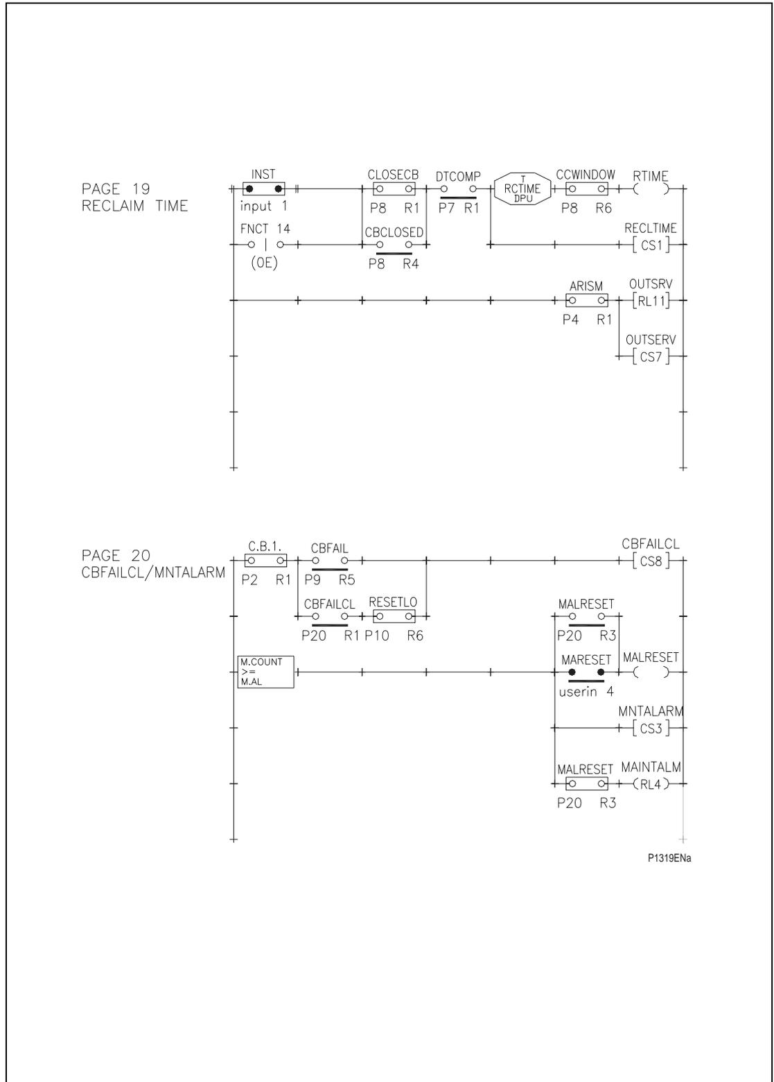
Figure 26. Scheme logic diagram : KAVR 100 (Drg No. 08 KAVR 100 01)
