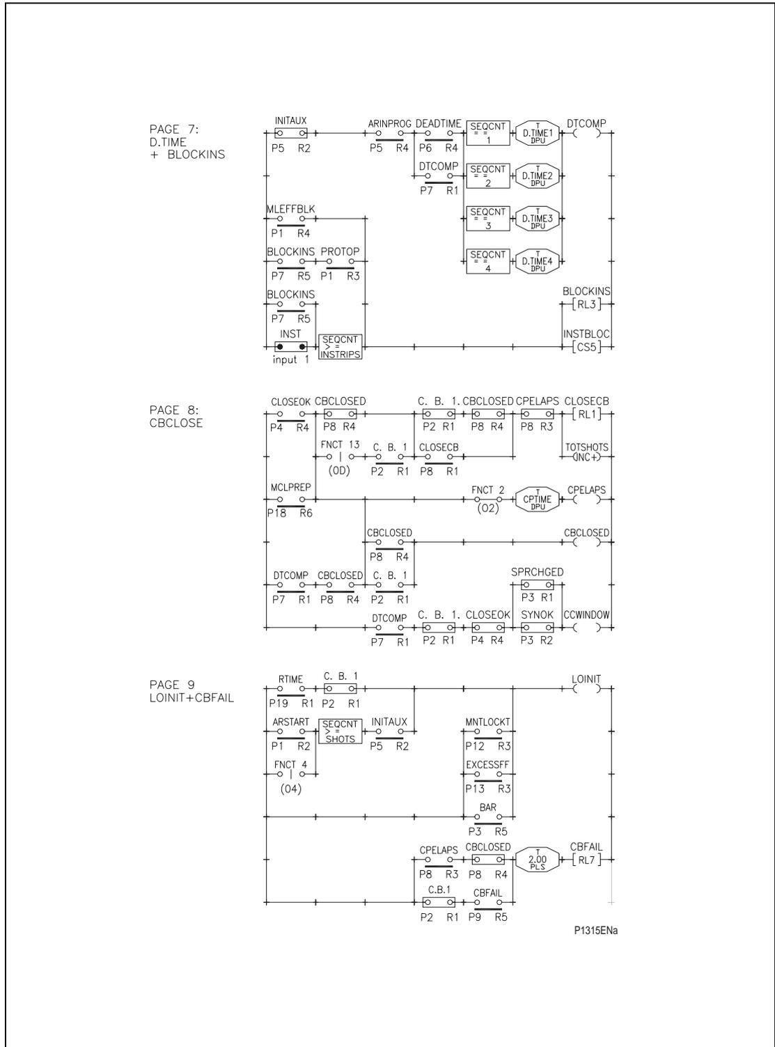
Figure 22. Scheme logic diagram : KAVR 100 (Drg No. 08 KAVR 100 01)
