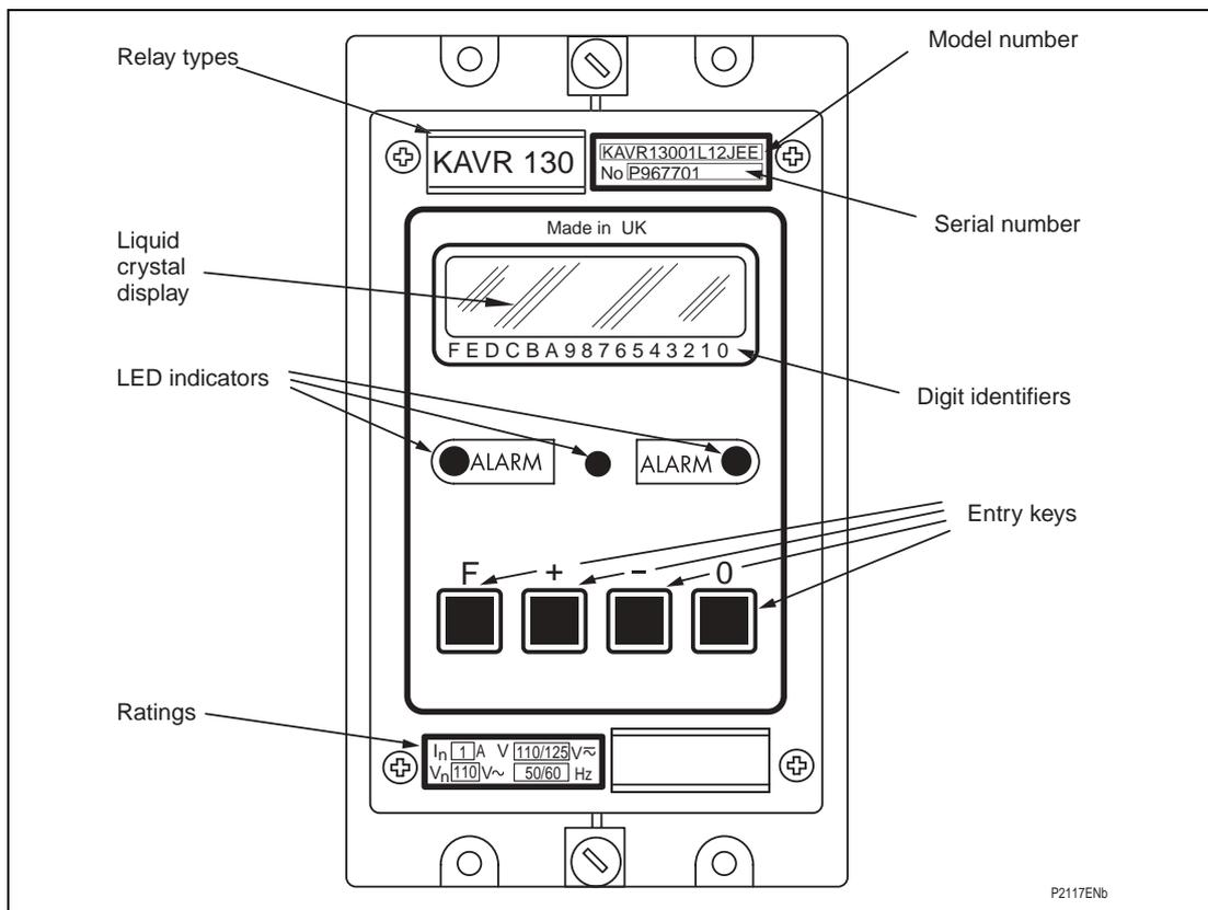
**Figure 5. Front plate layout**
