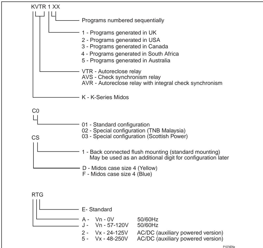
Note: Initial production relays will have the voltage rating marked as  $V_n = 110V$  and later models this will be marked 57 – 120V. The voltage rating and operational range is the same for both marked ratings and the only difference is in the label affixed to the relay.
