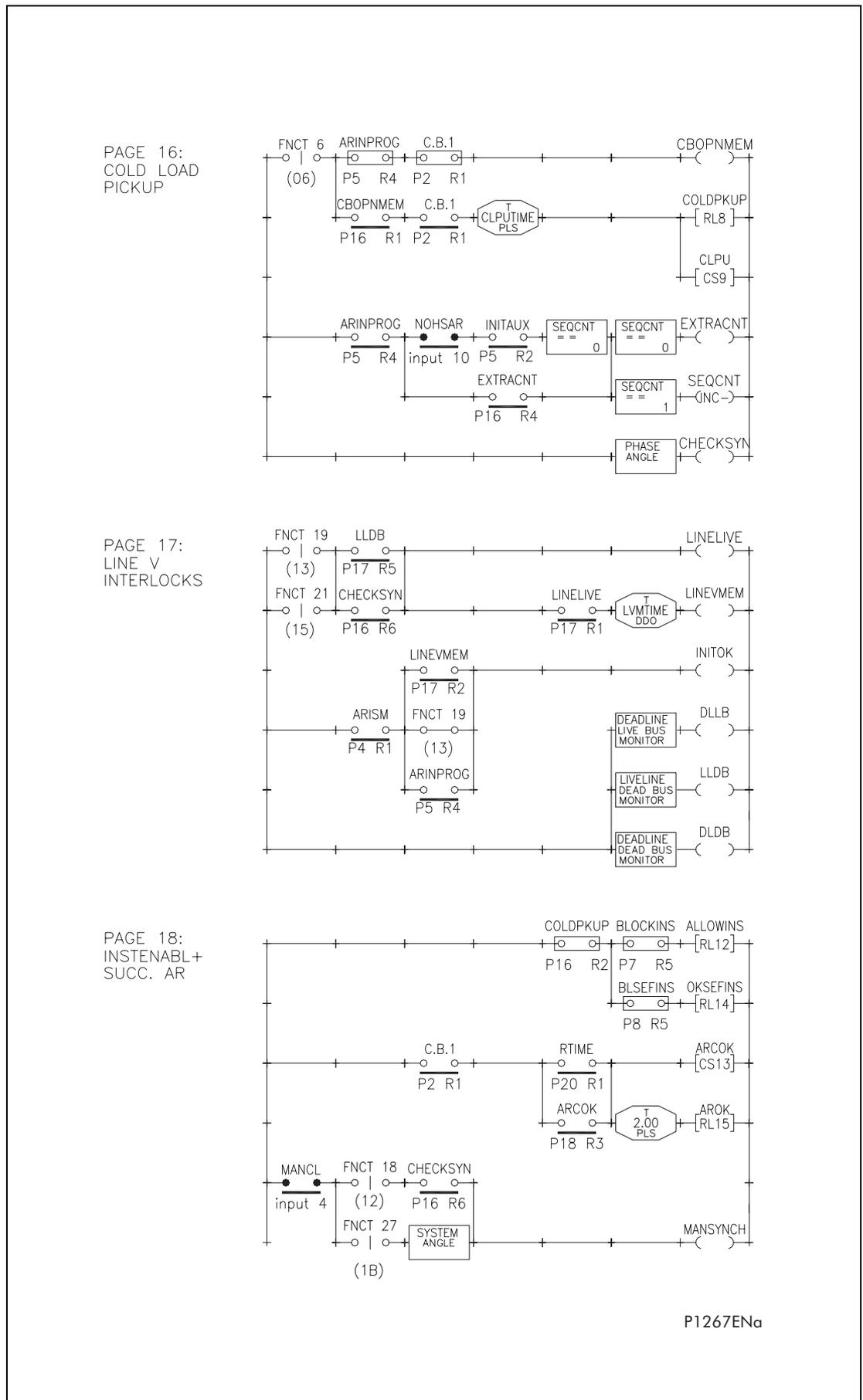
Figure 14. Scheme logic diagram : KAVR 100 (Drg No. 08 KAVR 100 01)
