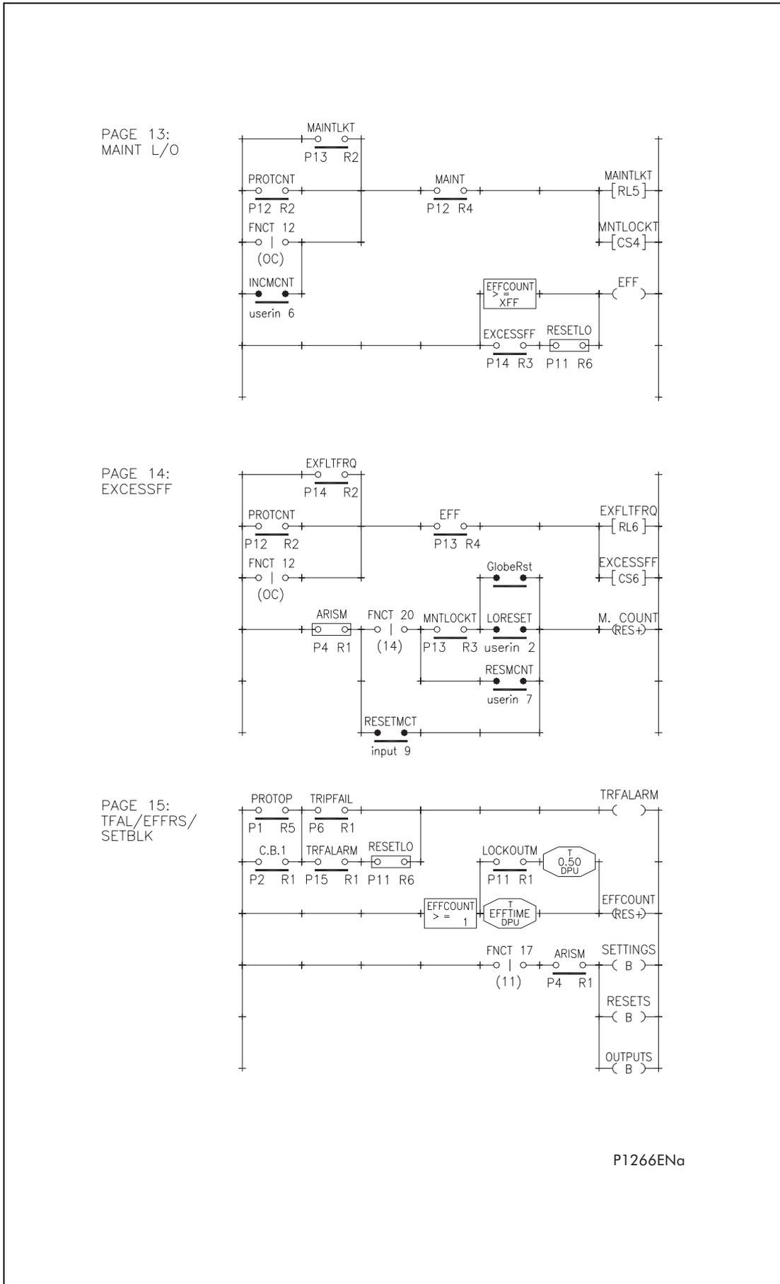
Figure 13. Scheme logic diagram : KAVR 100 (Drg No. 08 KAVR 100 01)
