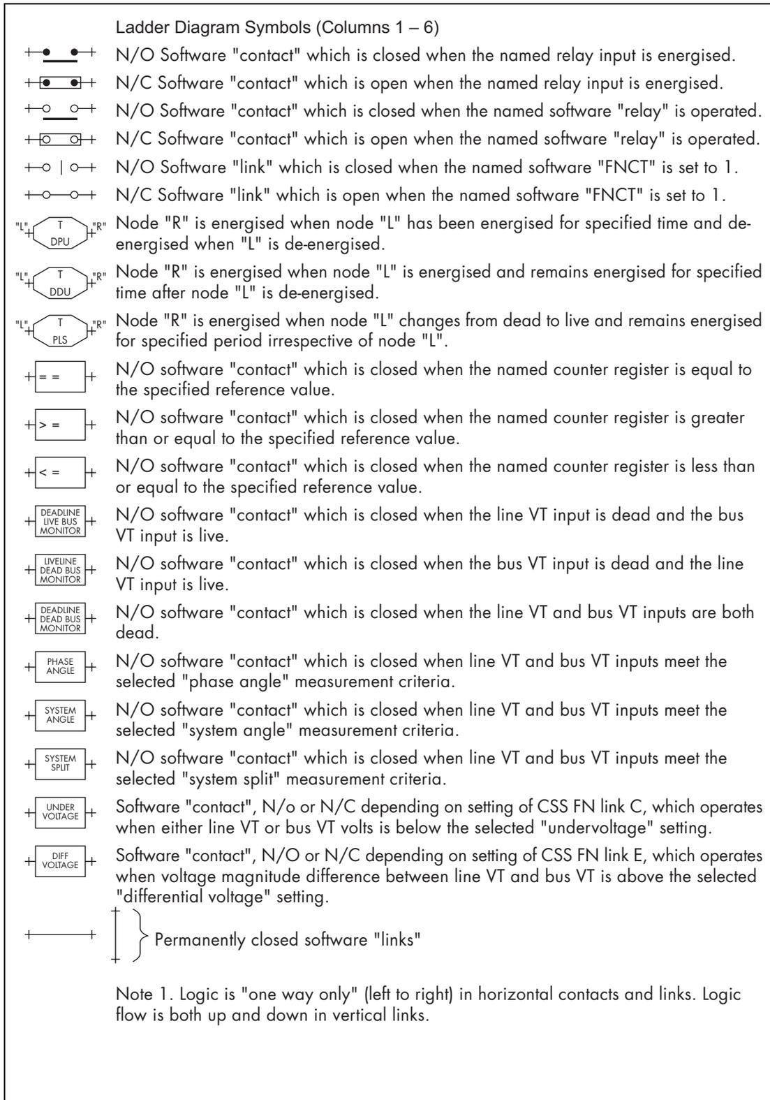
**Figure 29.** Ladder diagram symbols : (Drg No. 08 KAXX 00) sheet 1
