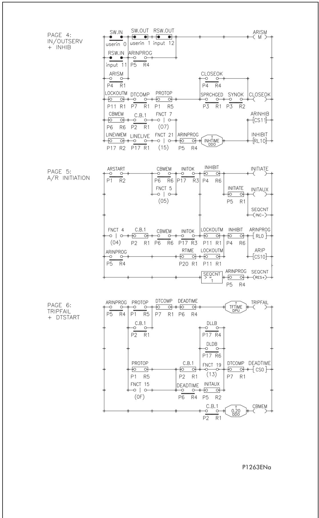
Figure 10. Scheme logic diagram : KAVR 100 (Drg No. 08 KAVR 100 01)
