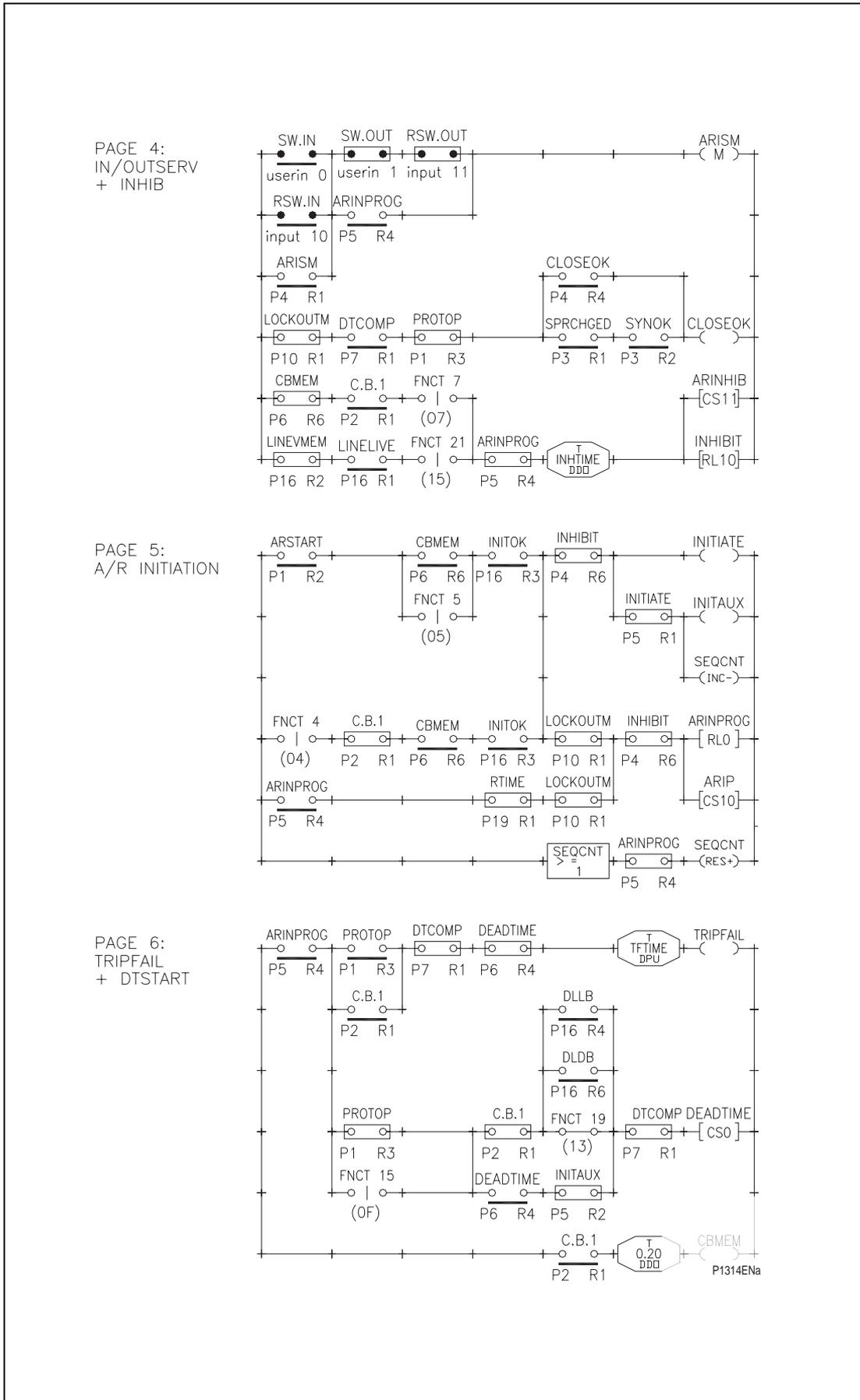
Figure 21. Scheme logic diagram : KAVR 100 (Drg No. 08 KAVR 100 01)
