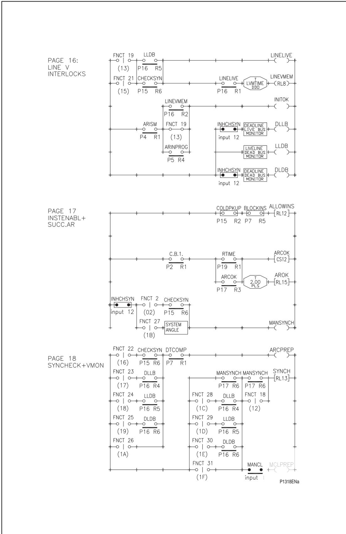
Figure 25. Scheme logic diagram : KAVR 100 (Drg No. 08 KAVR 100 01)
