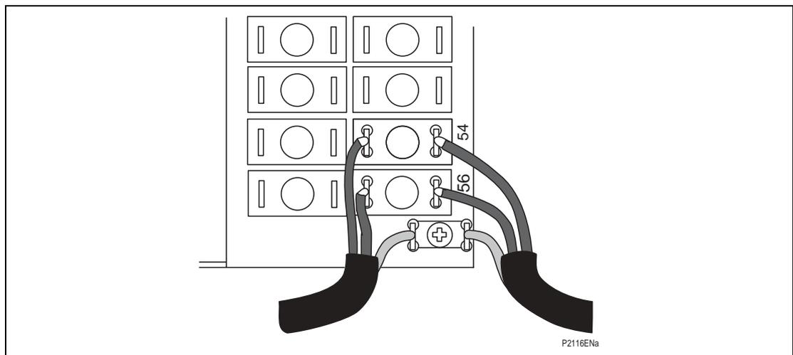
**Figure 4.** Terminal arrangement for communications
