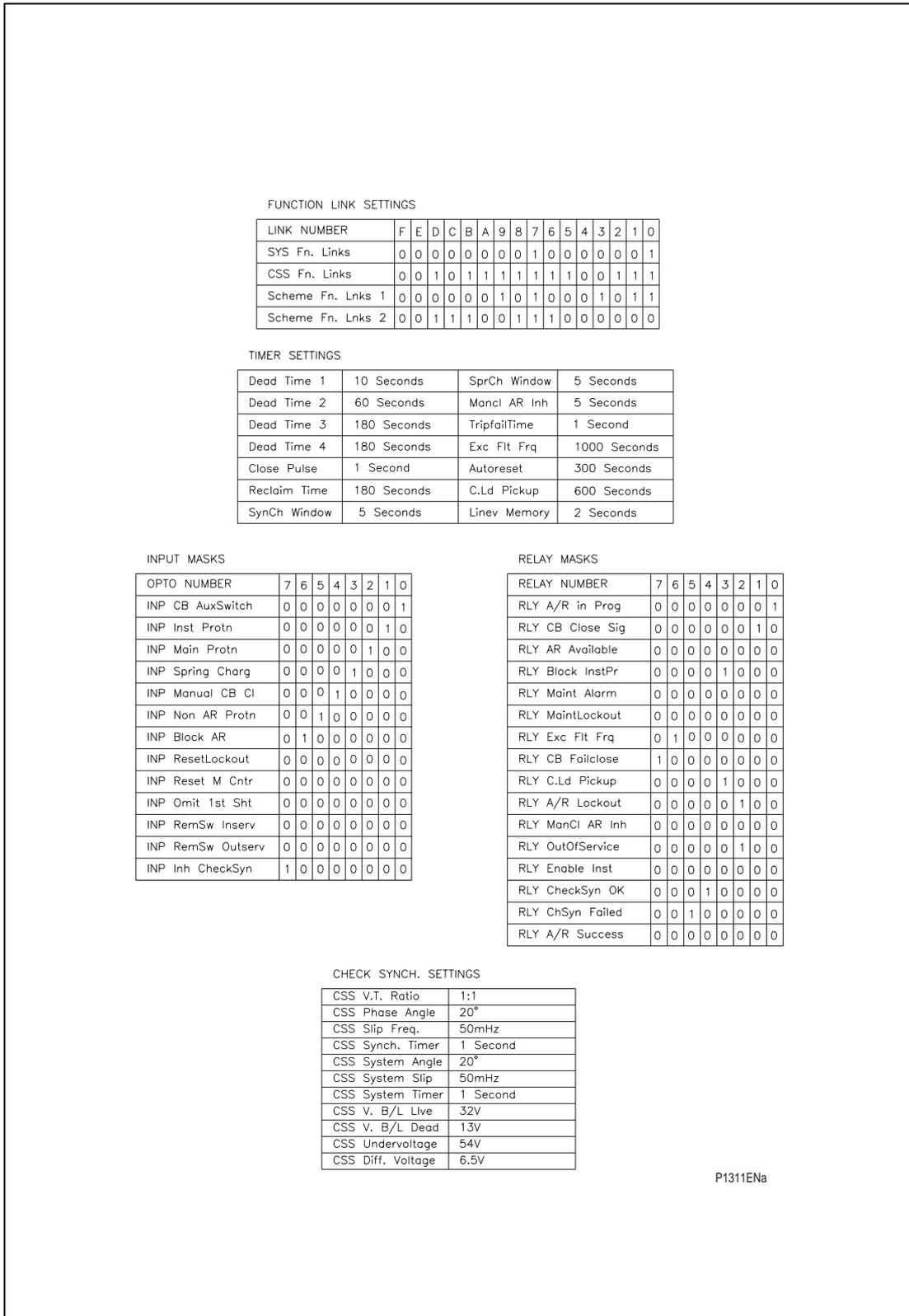
**Figure 27. Relay settings: KAVR 102 (factory default settings)
