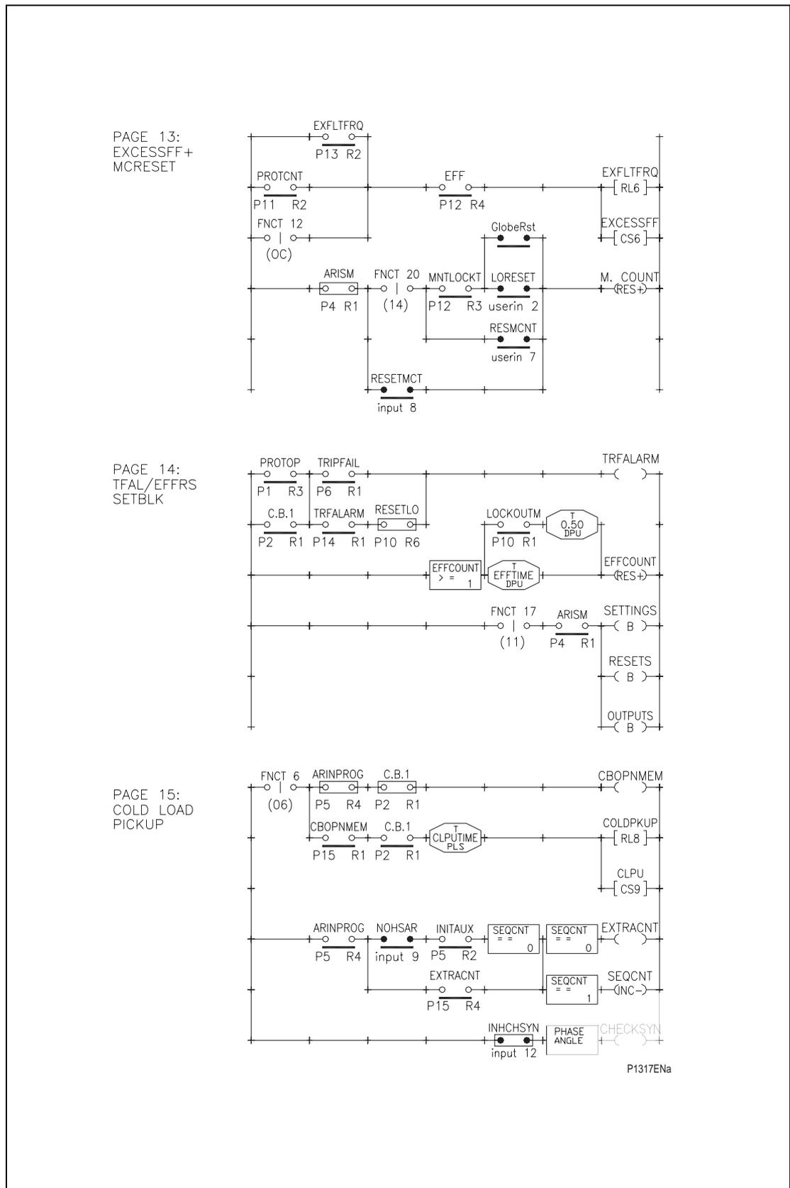
Figure 24. Scheme logic diagram : KAVR 100 (Drg No. 08 KAVR 100 01)
