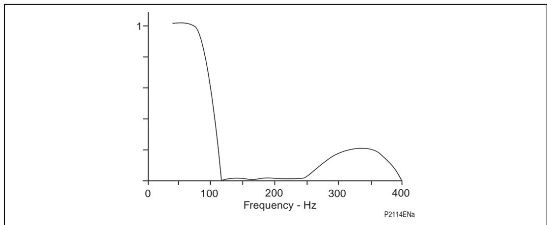
**Figure 2.** Frequency response for single voltage input
