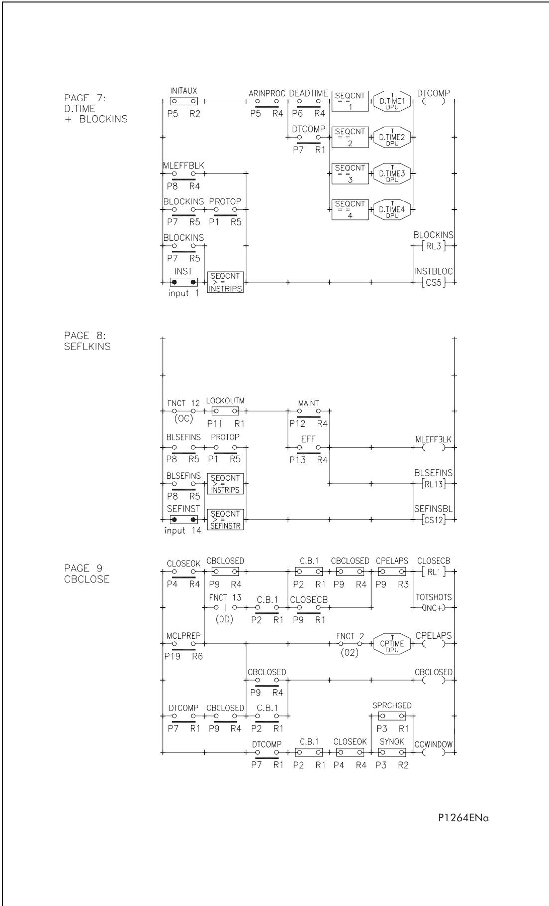
Figure 11. Scheme logic diagram : KAVR 100 (Drg No. 08 KAVR 100 01)
