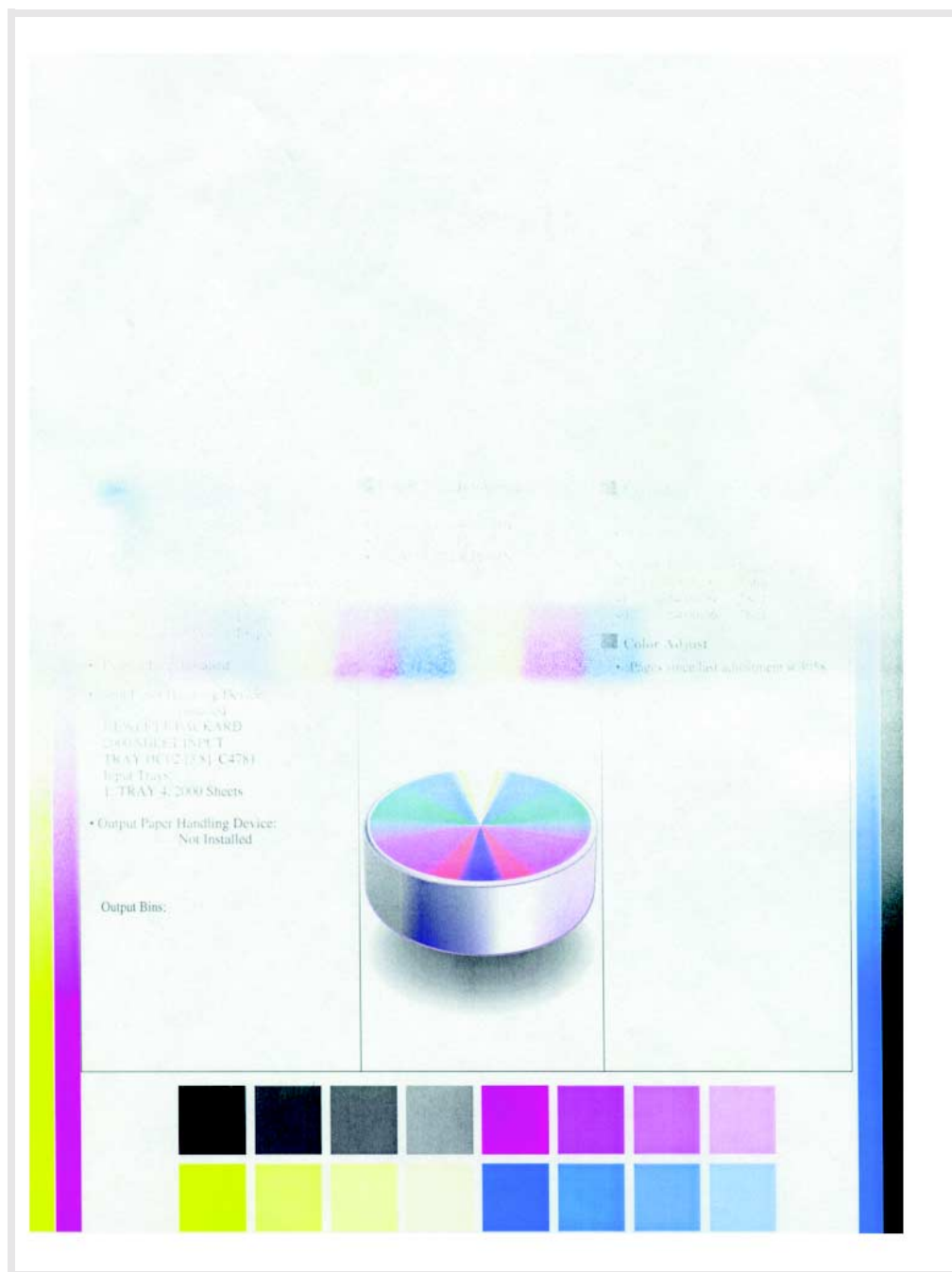
Fading resulting from broken transfer guide
