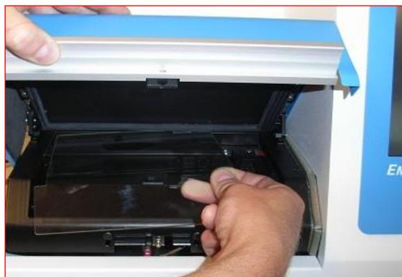
5. Remove slide holder by unscrewing the two bolts holding the slide holder in place. Pull gently towards you to remove the slide holder.
