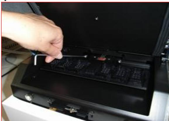
6. Clean internal surfaces and the slide holder (outside the device) with FertiSafe spray. Follow up with FertiSafe wipes: Wipe all internal surfaces and the slide holder with at least three wipes. Repeat until the wipes are not discolored.
