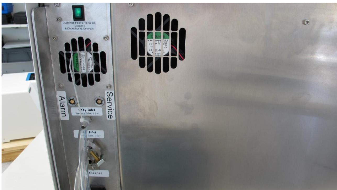
Attaching and securing CO<sub>2</sub> and N<sub>2</sub> supply through the appropriate and labeled inlets must be performed by Unisense FertiTech A/S personnel.
