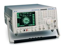
The 2968 TETRA Radio Test Set for comprehensive terminal and base station testing
