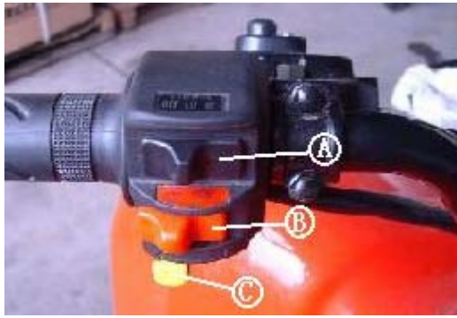
A. Light/Dimmer switch B. Engine stop switch C. Starting switch
