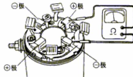
electric conduction capability for positive and negative poles
