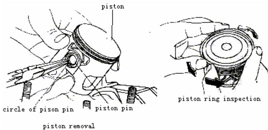
When inspecting piston and piston ring, first of all clean out carbon deposit. It is admitted to use old piston ring to do it. Never use steel wire brush to clean out them, otherwise it may damage its groove. Inspect the top and bottom surface of piston ring groove, replace piston if any damage or wry sharpennig appears (see fig.).
