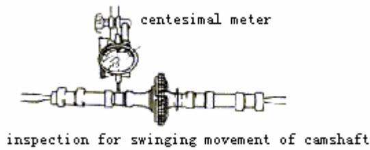
The combined clearance of camshaft is the difference between the inside diameter of axle bracket and the outside diameter of axle cervix. If bracket of camshaft is one part, you can measure it with centesimal meter.
