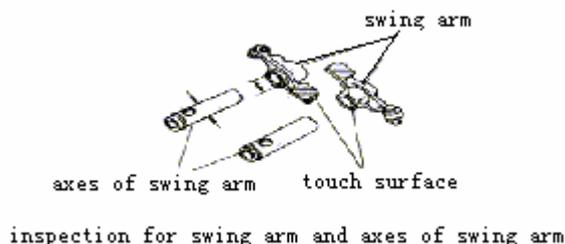
Measure the inside diameter of swing arm and the outside diameter of sliding sect of swing arm axes, at the same time calculate the clearance between swing arm and its axes. If the dimension is out of its limit, replace it.
