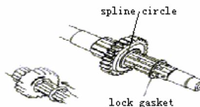
4. Assemble bush or gear with oil hole; keep the hole dead against the oil hole of axis (see fig.).
