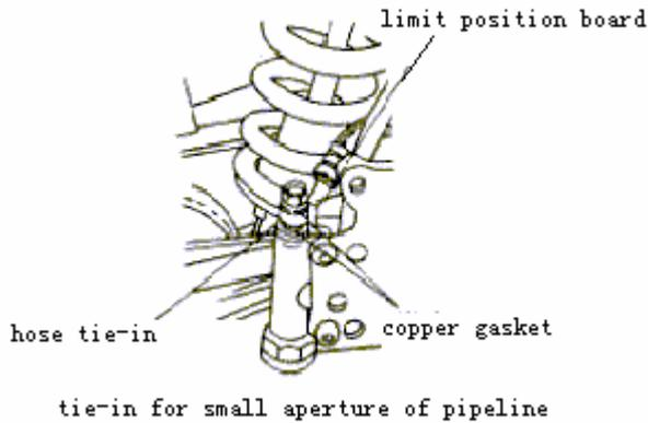
tie-in for small aperture of pipeline
