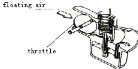
block throttle valve starting system
