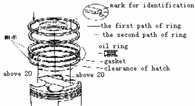
piston ring assembly for four-stroke engine
