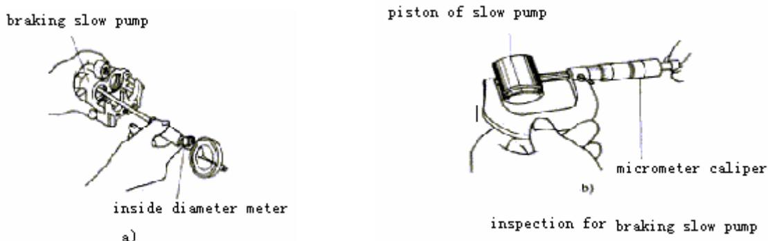
Disassembled configuratin of braking main pump as shown, inspect its body and piston after disassembling it including damage, scratch and step abrasion on its surface, and replace them if necessary. Measure main pump's inside diameter for several times with centesimal meter and measure the outside diameter of piston of main pump for several times with micrometer as shown. If one diameter is out of its limit, replace it.
