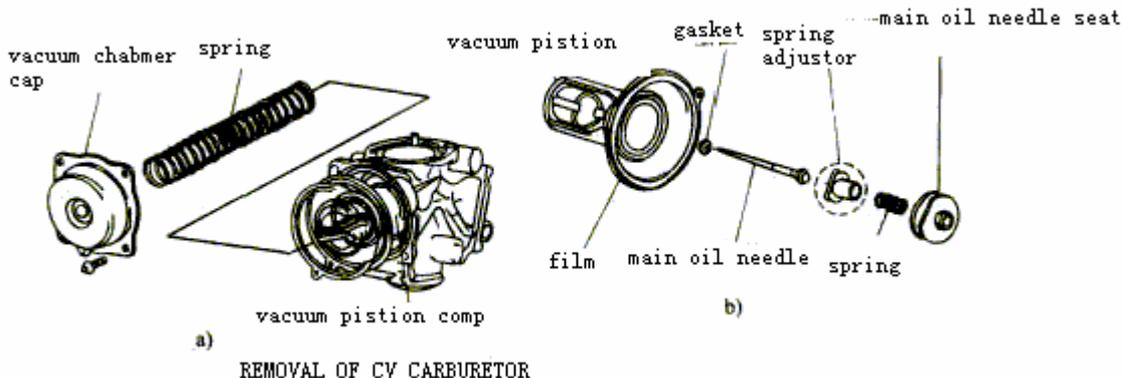
For plug throttle its structure is the following figure: after removing it, inspect whether its fluctuating movement is smooth and main oil needle is abraded or not.
