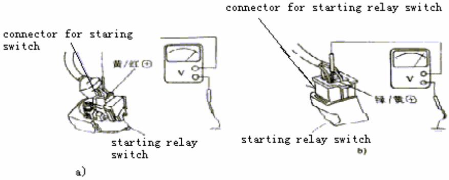
inspect the voltage of starting switch
