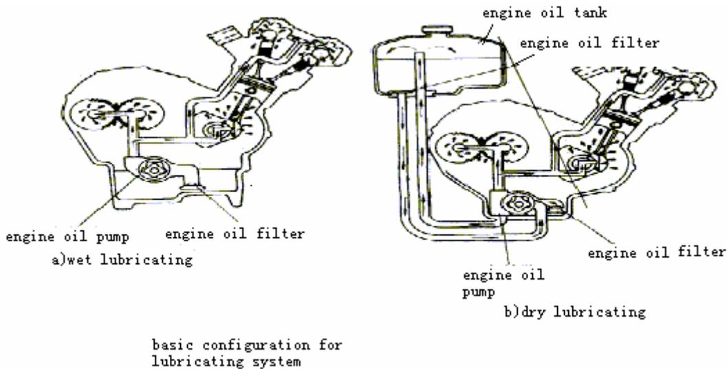
For 2-stroke engine it uses the inside of crankcase as inspiration and adding pressure chamber, so it cann' t install bottome shuck of engine oil like 4-stroke engine. Mis engine oil and gasoline and use atomized lubrication to lubricate cylinder and rotating part of crankshaft bearing. For QJ 2-stroke motorcycle it mostly uses separated lubricating mode.
