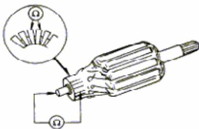
inspection for electric conduction capability of armature
