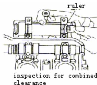
Replace cam if combined clearance is out of its limit, at this time you need to calculate whether the clearance is at the standard range. If not, replace cam, bracket of camshaft and cylinder cap.
