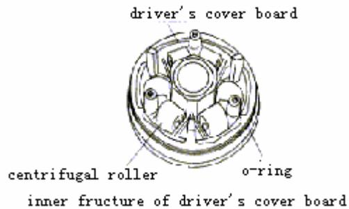
Insepect driver' s centrifugal roller, cover board and bush (see fig.) . If damaged or declining abraded, replace it. Measure outside diameter of centrifugal roller and bush, inside diameter of cover board. replace it if measured diameter is over its limit.
