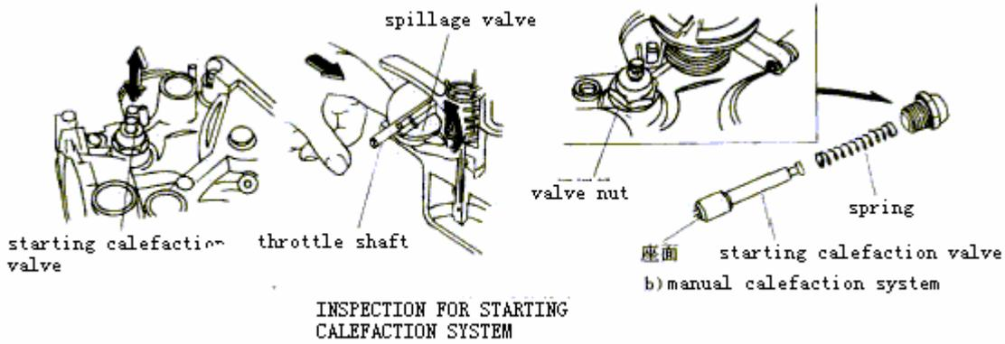
For throttle, you also need to inspect whether moving shaft becomes flexible or not, pull spillage valve of throttle with finger to inspect whether it can be opened or closed. For manual starting concentration valve, you also need to disassemble it and inspect its surface, if there is damage, leaning abrasion or sidestep fray on the seat of valve, replace it.
