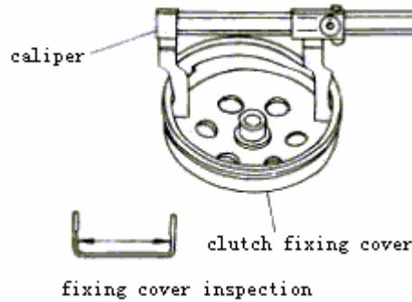
Measure outside diameter of driven wheel and the touching part of driven left disc, replace it if measured diameter is below its limit. Measure inside diameter of driven wheel left disc; replace it if measured diameter is below its limit. Inspect guide pin groove on driven wheel disc; replace it if abrasion like side step appears.
