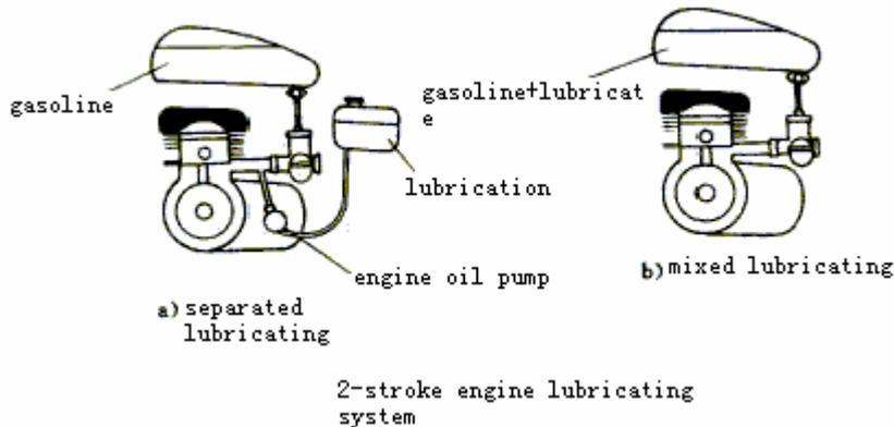
Engine oil pump is main part of lubricating device, for 4-stroke engine its engine oil pump uses trochoid gear pump and for 2-stroke engien it uses plug engine pump.
