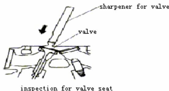
When inspecting valve pipe, insert a sword into the pipe to clear out carbon deposit. See picture: turn right to insert sword into or take it out of the pipe to avoid damaging inside surface of pipe. Measure the inside diameter of valve pipe with centesimal meter, and calculate the distance from valve handspike to pipe. If measured distance is over its limit, replace it.
