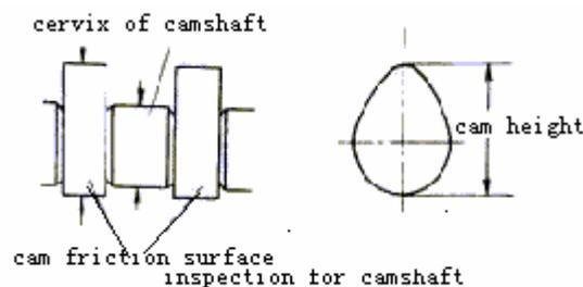
Including the following outer dimension: outside diameter of axes cervix, height of
