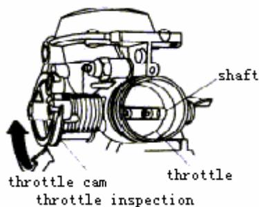
For CV type of carburetor its removal structure is the following figure: after removing it inspect whether vacuum tube can rotate smoothy in carbutetor. Inspect whether there
