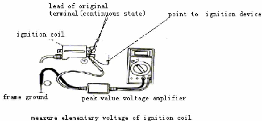
When using peak vottage to inspect ignition coil, take down plug from CDI device and connect the end of ignition coil with leak voltage amplifier. If the gap of spark plug is proper, turn crankshaft through starting motor, and then read the leak voltage of ignition coil.
