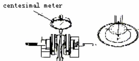
inspection for radial movement of big top of connecting rod
