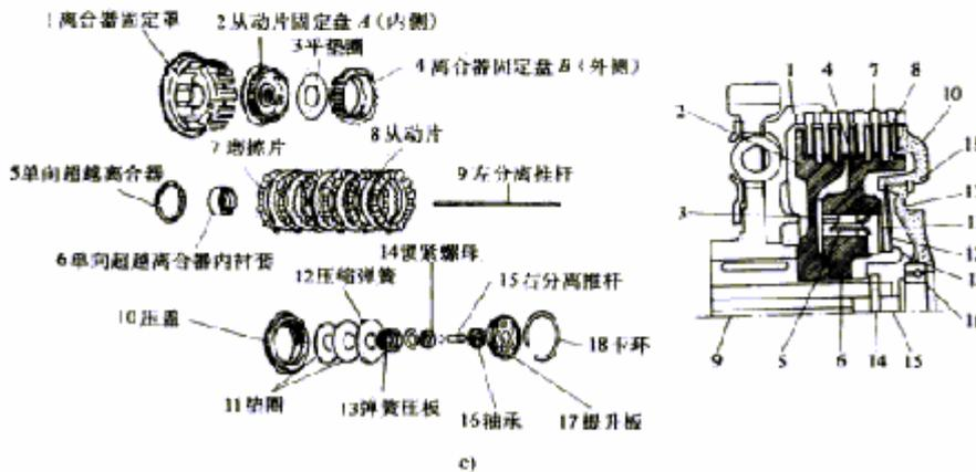
图 8-213 structure of wet multiplate manual clutch
