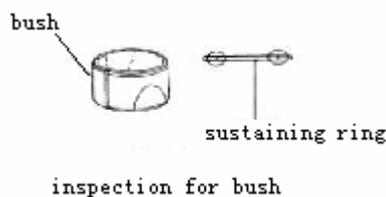
Other parts of front fork (see the following fig.): bushing, piston and so on. Inspect every part to see whether there is scratch, bend, crack or abrasion etc. or not, replace them if necessary.
