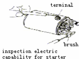
Measure the distance of brush (see fig.), inspect whether the degree of abrasion is over its limit or not, replace it if it is.
