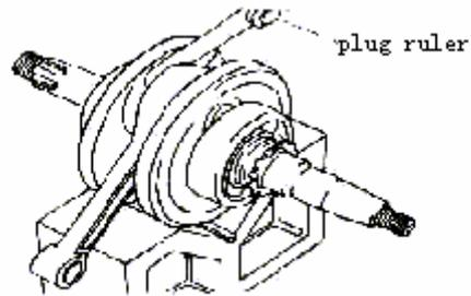
crankshaft and connecting rod inspection
