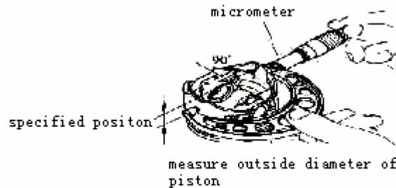
Inspect the hole of piston pin (see fig.): measure it in direction X AND Y, regard the maximum as its inside diameter. Replace it if the maximum is over its limit.
