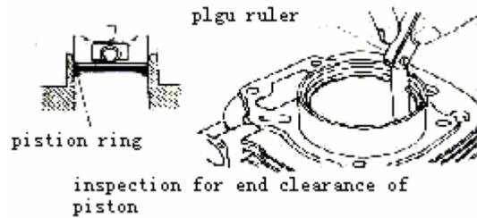
If measured end clearance or side clearance is over its limit, replace piston ring.
