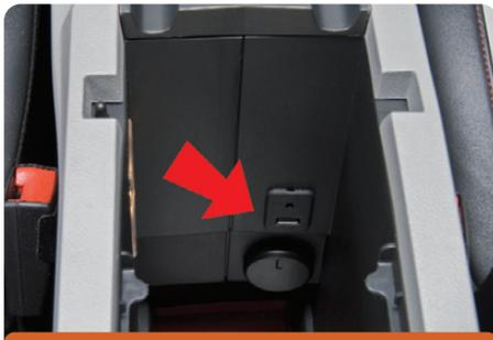
Some programming can be performed through the vehicle's USB port.
