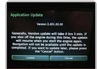
Follow the on-screen prompts after inserting the USB flash drive in the vehicle's USB port.
