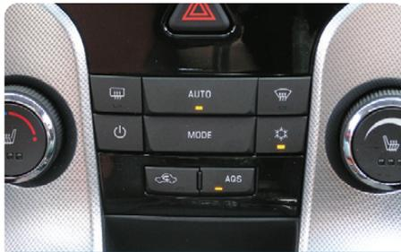
The automatic climate controls have an Air Quality Sensor.
