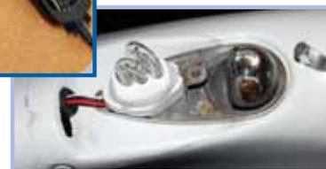
1. Remove the position light lens retainer being careful not to drop the red or the green lens.
