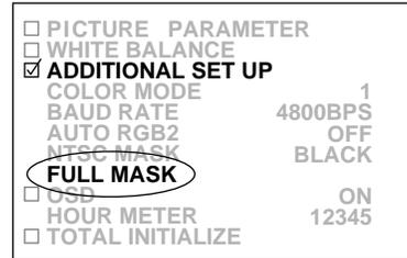
4. Select "WHITE" using the ↑ or ↓ key and press the SET key. Then the display immediately changes to the full-color mask screen.
