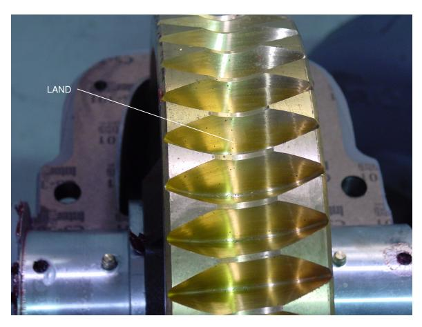
Check gear wear by removing the cover and visually inspecting the bronze gear. If the gear is worn such that there is no visible land on the throat of the gear between the gear flanks as shown in picture above the gear should be replaced.
