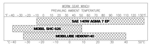
All oils must meet MIL-PRF2105E standards. Substitution from a reputable manufacturer is allowed as long as type and grade are maintained.
