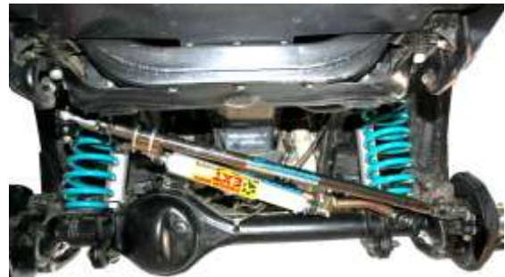
Figure 2: Correctly Fitted Drag Link
