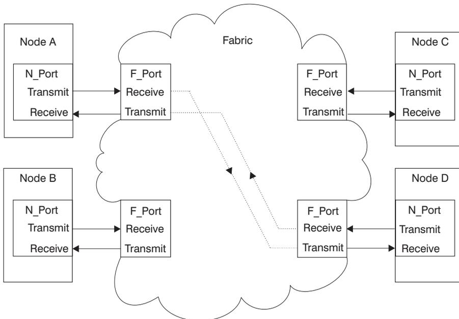
Figure 4. Fabric Topology Showing Node A Currently Connected to Node D
