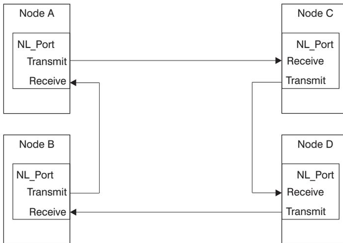
Figure 2. Arbitrated Loop with Four Nodes
