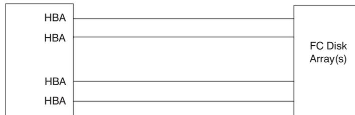
Figure 7. Example of a Point-to-Point Configuration
