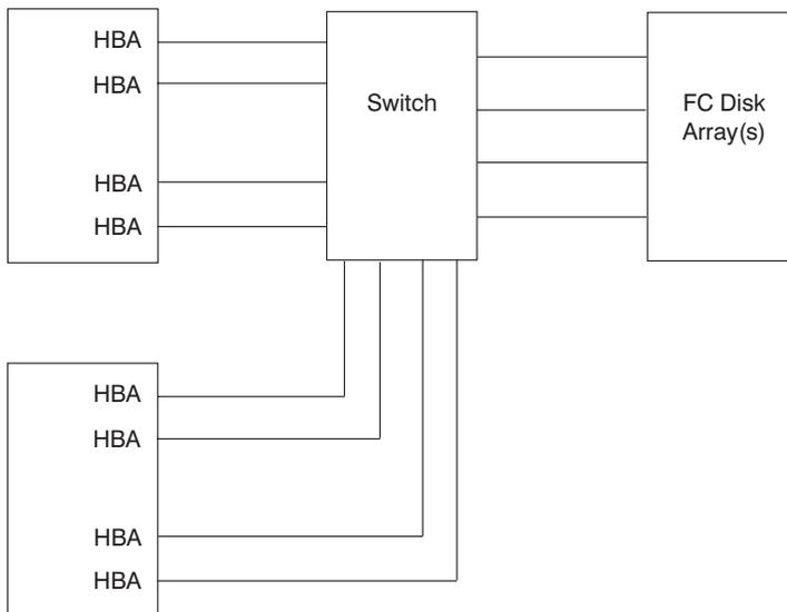
Figure 12. Example of a Switch Configuration With Two Host Systems Attached
