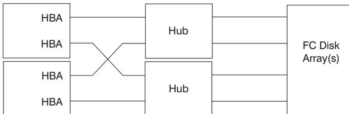
Figure 9. Example of a Hub Configuration With Two Host Systems and Two Hubs
