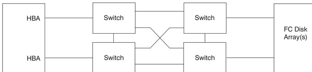
Figure 16. Example of a High Availability Configuration With a Single System and Four Cascaded Switches
