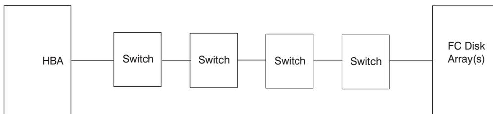
*Figure 14. Example of a Configuration With Four Cascaded Switches*
