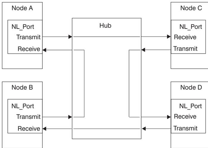
Figure 3. Arbitrated Loop Using a Hub
