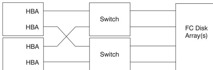
Figure 15. Example of a High Availability Configuration With Two Systems and Two Switches
