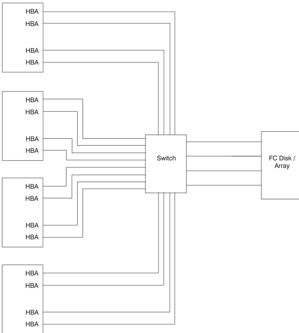
Figure 13. Example of a Switch Configuration With Four Host Systems Attached
