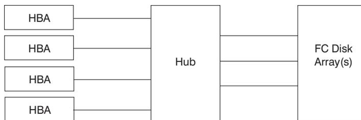
Figure 10. Example of a Hub configuration With four Host Systems and One Hub
