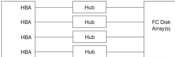
Figure 8. Example of a Hub Configuration With One Host System and Four Hubs
