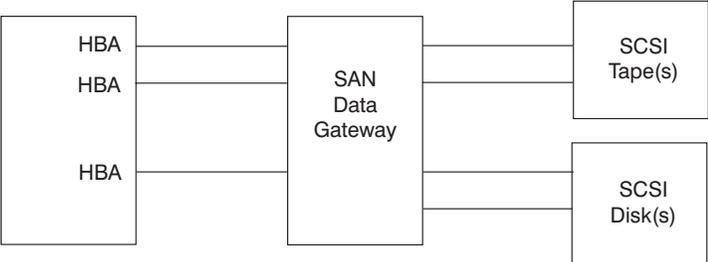
Figure 17. Example of a SAN Data Gateway Configuration With One Host System Attached
