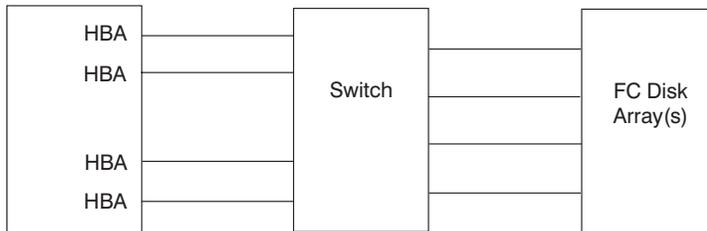
Figure 11. Example of a Switch Configuration With One Host System Attached
