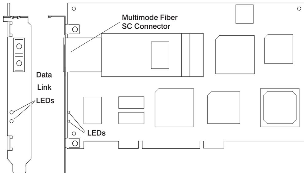
Figure 5. Gigabit Fibre Channel PCI Adapter
