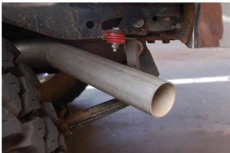
pan over to the passenger's side. Merge it and the passenger bank into a Y-pipe and send it out as a single circuit down the passenger side, up over the axle out exiting at the rear.
