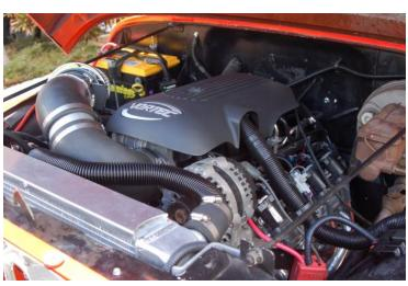
If you are wishing to run an onboard air compressor without losing A/C, we recommend that you install our Air Conditioning Relocation kit, which provides a new compressor and mounts it up at the passenger side head location on Gen. III+ engines.
