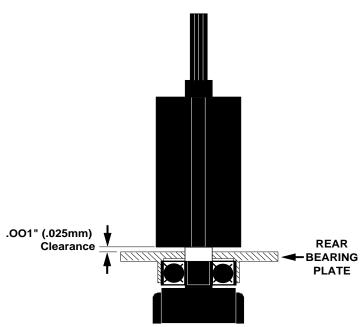
After final assembly of the motor unit has been completed, inspect it to ensure that the rotor does not rub the front bearing plate.
