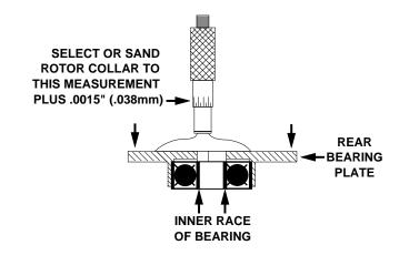
Assemble the collar, rotor bearing, bearing plate, and governor assembly (left hand threads) to the rotor. Check clearance between rear bearing plate and rotor. The clearance should be .001" (.0254mm) after the governor is tightened to the rotor.
