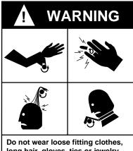
Follow good machine shop practices. Rotating shafts and moving components can entangle and entrap, and can result in serious injuries. Never wear long hair, loose-fitting clothes, gloves, ties, or jewelry when working with or near a drill of any type.
