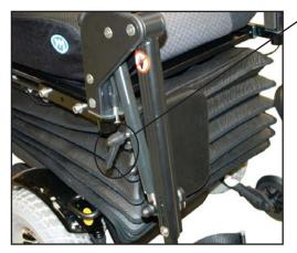
To adjust the footplates up and down, loosen the clip.
