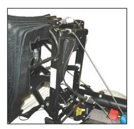
You can now tilt the seat forward for access to the batteries.
