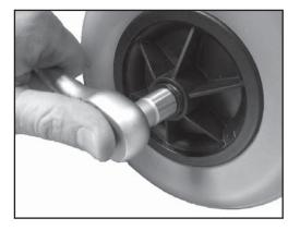
Pivot wheel Undo and remove the middle nut.
