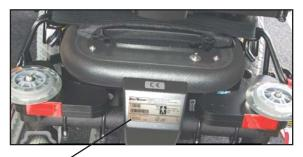
Position of serial number plate on vehicle.
