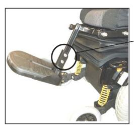
To adjust the footplate up and down, undo the screws shown here. You can now adjust the footplate to the required height.
