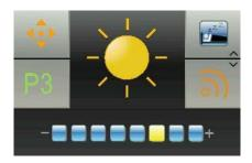
Press the arrow up / down until the sun i shown i the centre. Push the joystick forward to enter the settings. Use the Select button or joystick right / left to change the brightness.
