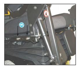
You can adjust the footrests forwards and back. This can be done by undoing the two screws indicated.
