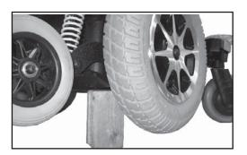
Jack up the MC Concept onto a block of wood so that the wheels are clear of the floor/surface.
