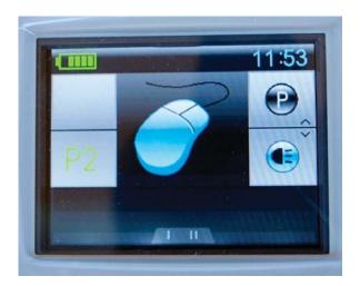
Use arrow up / down to find the mouse icon. As long as the mouse is blue, it is not active. Activate by pushing the joystick forward. Now the mouse turns green.
