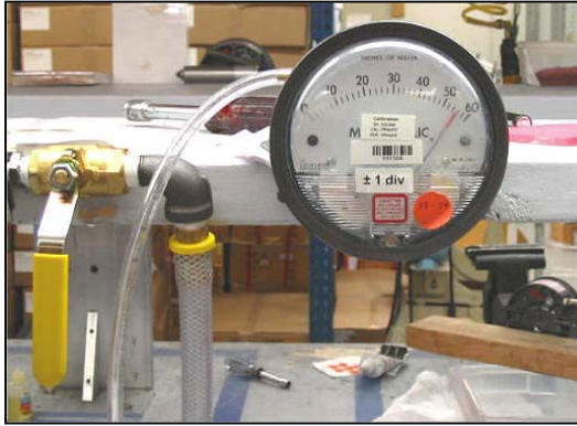
Figure 32. Magnehelic Gauge Connection to Hose Barb
