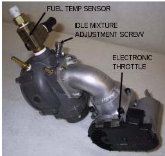
Figure 12. Idle Mixture Adjustment Screw
