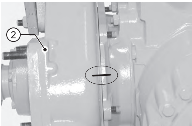
FIGURE 3: DIRECTLY FLANGED VERSION ONLY Mark the housing position before removing.
