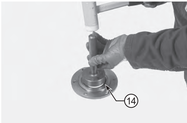
FIGURE 14: Remove the cover sealing ring (14).
