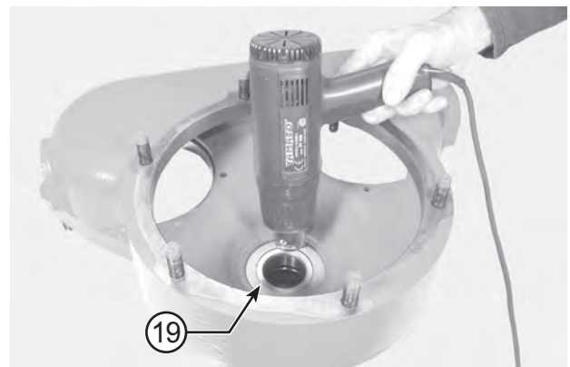
FIGURE 31: Heat the inner bearing (19) to about 100 C°.
