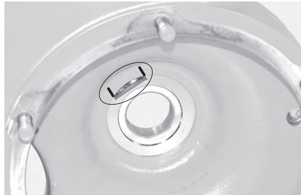
FIGURE 24: Verify the oil shield plate (18) position marked during disassembly.
