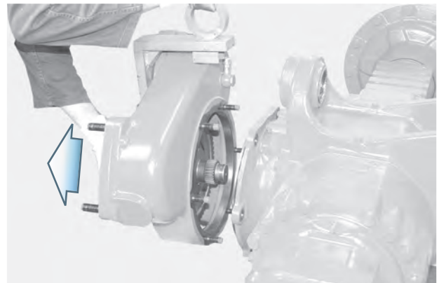
FIGURE 5: DIRECTLY FLANGED VERSION ONLY Disjoin the entire reduction unit (2) from the axle and place it on a bench.
