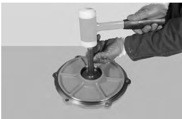
FIGURE 15: Move the bearing to the limit stop by hammering lightly all around the edge.
