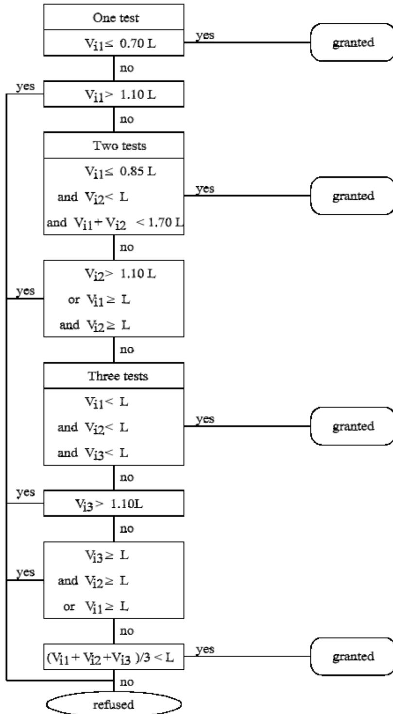
5.3.2. Type II test (Carbon monoxide emission test at idling speed)
