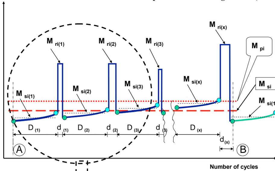
**Figure 8/2:** Parameters measured during emissions test during and between cycles where regeneration occurs (schematic example)
