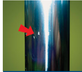
Damaged chrome plating
