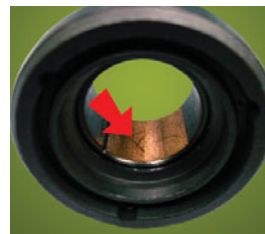
Damaged oil seal
