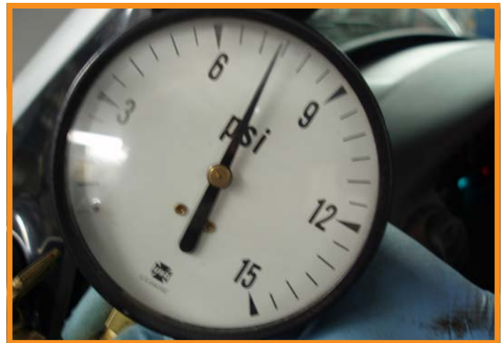
Photo 4: A snap-throttle test on this converter revealed an exhaust restriction that had passed conventional testing methods.
