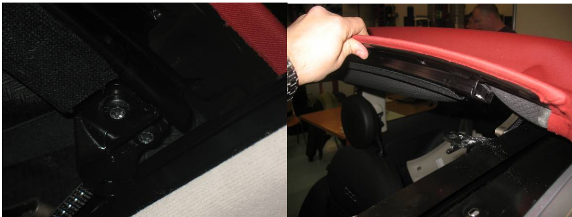
Canvas fastening screws to the first front rib, on the left side.
