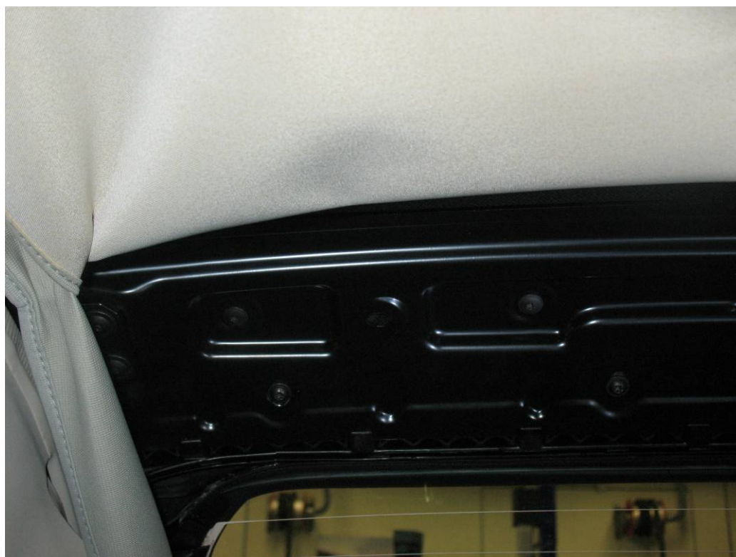
Screws securing the spoiler to the cross member.
