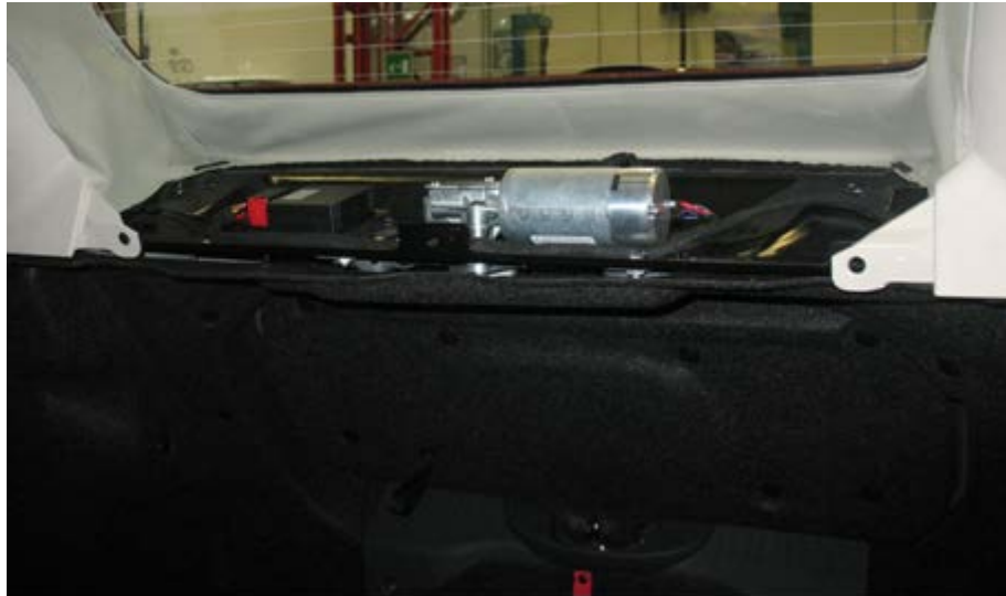
RCU control unit and motor.
